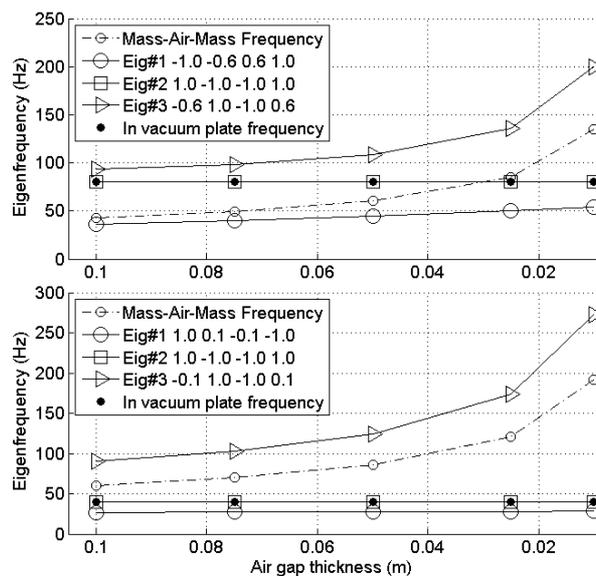
**Figure 3.** First eigenfrequencies predicted by model in Figure 1 for a double leaf HB structure considering two panels' thickness, providing structural masses of 500 (top) and 250 (bottom) Kg, for different thicknesses of the air gap between the panels.
