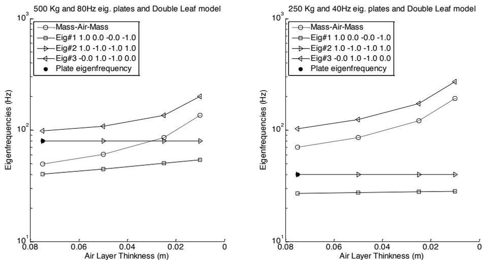
**Figure 4.** Eigenfrequencies of double leaf structures through a model considering each panel as two degrees of freedom systems and the air both as a massless and distributed mass stiffness element for two structures: structural panels with 80 Hz (left) and 40 Hz (right) as fundamental frequency.
