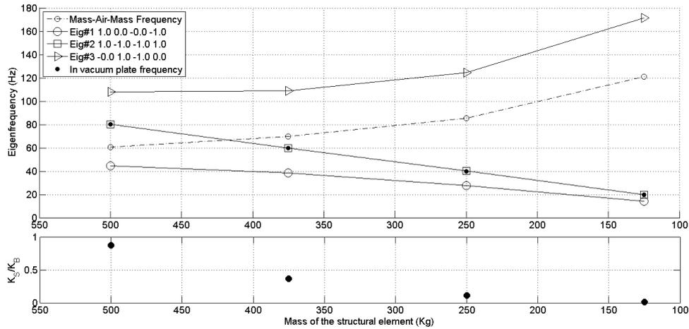
**Figure 2.** Top: Eigenfrequencies corresponding to model in Figure 1 for several cases of mass and in vacuum eigenfrequencies for the structural elements; in vacuum structural fundamental frequency and ideally predicted *mass-air-mass* resonance. Bottom: ratio between structural and fluid stiffness.
