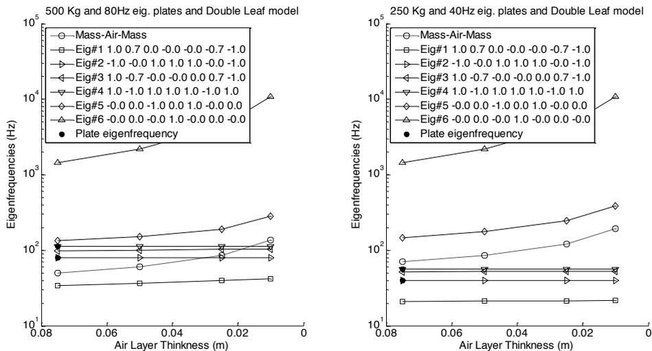
**Figure 8.** Eigenfrequencies of double leaf structures through a model considering each panel as three degrees of freedom systems and the air as a single degree of freedom system for two structures: structural panels with 80 Hz (left) and 40 Hz (right) as fundamental frequency.
