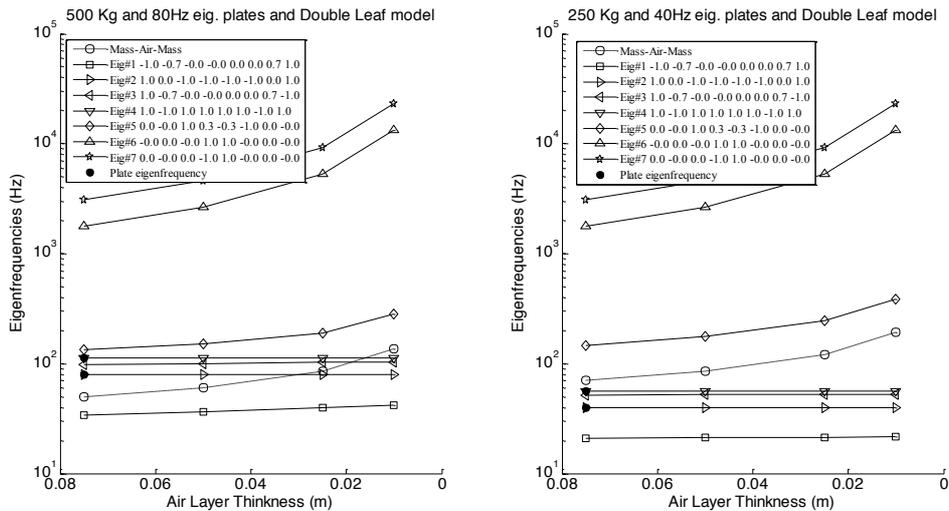
**Figure 7.** Eigenfrequencies of double leaf structures through a model considering each panel as three degrees of freedom systems and the air as a two degrees of freedom system for two structures: structural panels with 80 Hz (left) and 40 Hz (right) as fundamental frequency.
