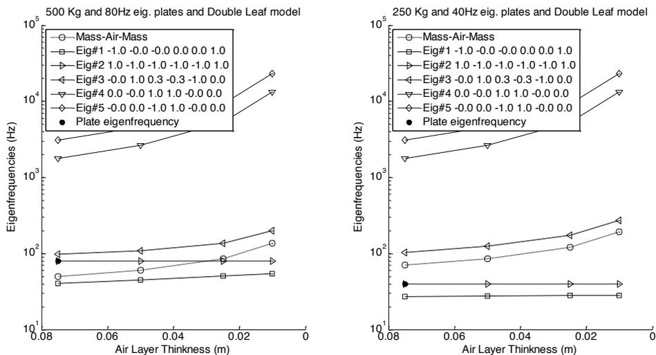
**Figure 6.** Eigenfrequencies of double leaf structures through a model considering each panel as two degree of freedom systems and the air as a two degrees of freedom system for two structures: structural panels with 80 Hz (left) and 40 Hz (right) as fundamental frequency.
