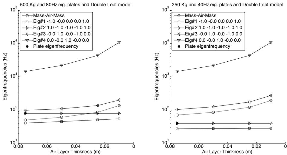
**Figure 5.** Eigenfrequencies of double leaf structures through a model considering each panel as two degrees of freedom systems and the air as a single degree of freedom system for two structures: structural panels with 80 Hz (left) and 40 Hz (right) as fundamental frequency.
