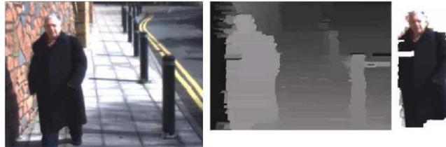
Fig. 4. Obstacle detection based on depth map thresholding.
