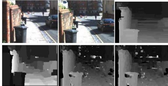
Fig. 2. First row: a pair of stereo images and depth estimation based on dynamic programming using 1D optimisation; second row: results obtained from belief propagation, sum of absolute difference with winner-take-all optimisation, and sum of squared difference with iterative aggregation.
