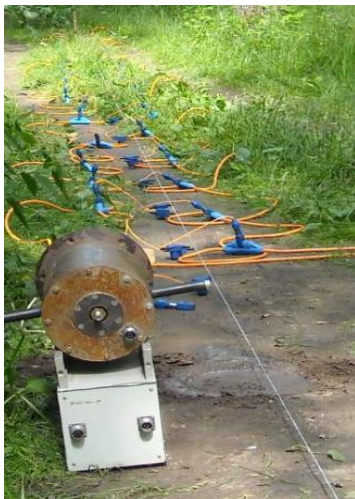
Figure 1. The source and receiving array (on the left). General scheme of measurements (on the right). Small circles and rectangles correspond to the positions of vertically and horizontally oriented geophones respectively, a large circle – to the position of the source.
