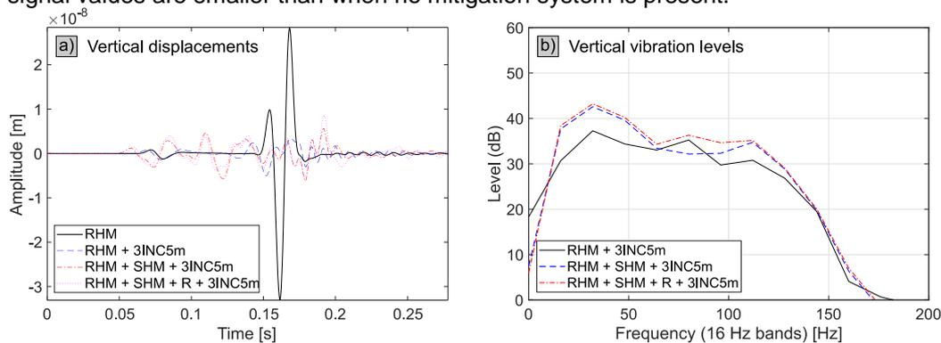
Figure 5 – a) vertical amplitudes over time and b) vertical vibration levels with inclusions
