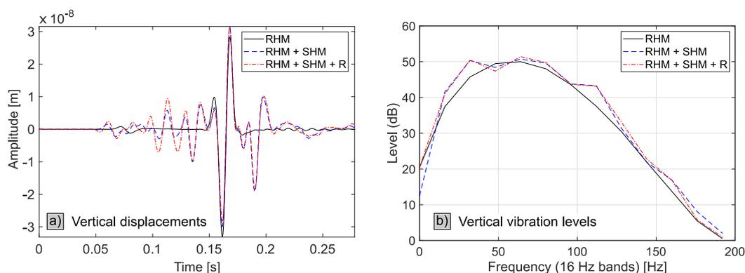
Figure 3 – a) vertical amplitudes over time and b) vertical vibration levels
