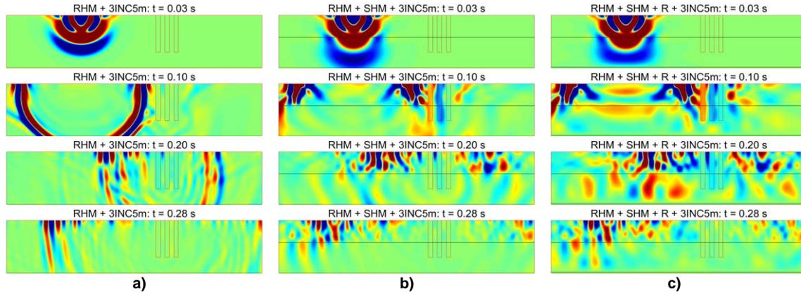
Figure 6 – Propagation over time (vertical displacements) with 5 m depth inclusions in a) reference medium, b) (reference + stiffer) medium and c) (reference + stiffer) medium + rock
