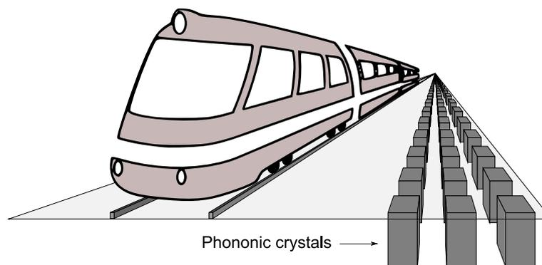
Figure 1 – New mitigation devices (phononic crystals)
