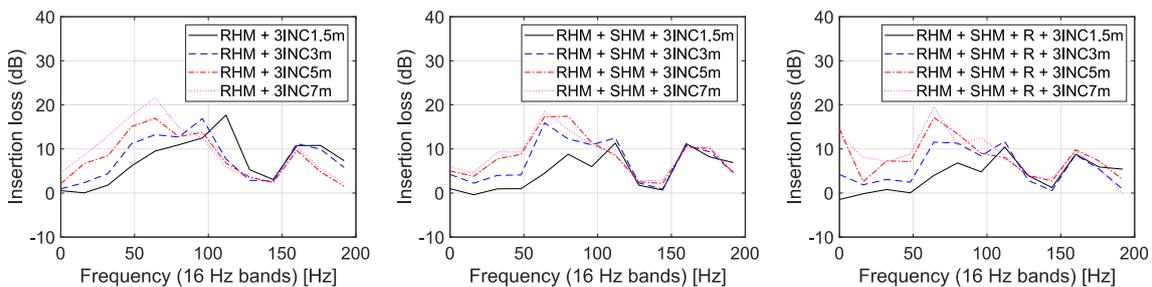
Figure 7 – Insertion loss of mitigating devices in different stratified media
