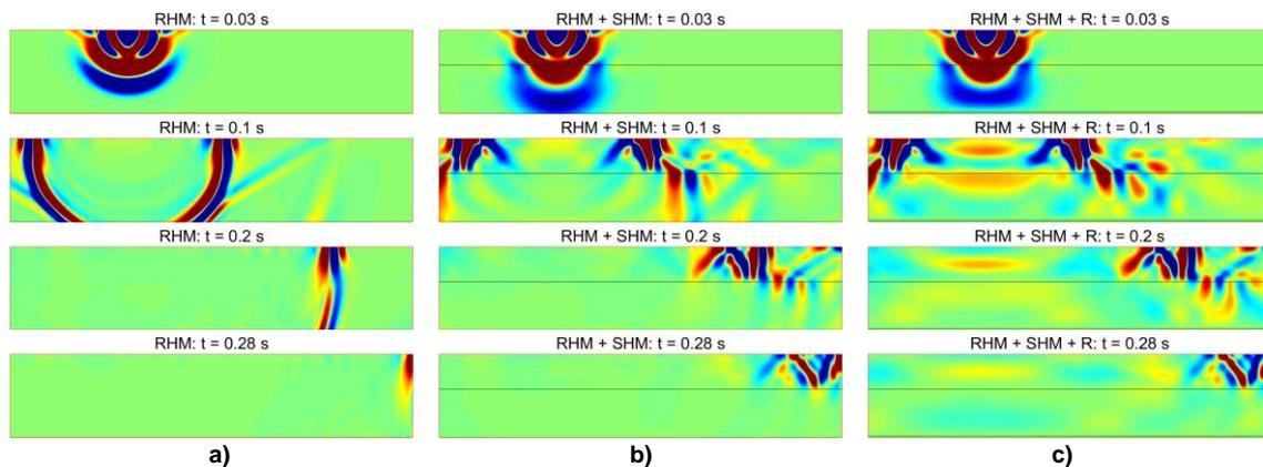
Figure 4 – Propagation over time (vertical displacements) in a) reference medium, b) (reference + stiffer) medium and c) (reference + stiffer) medium + rock
