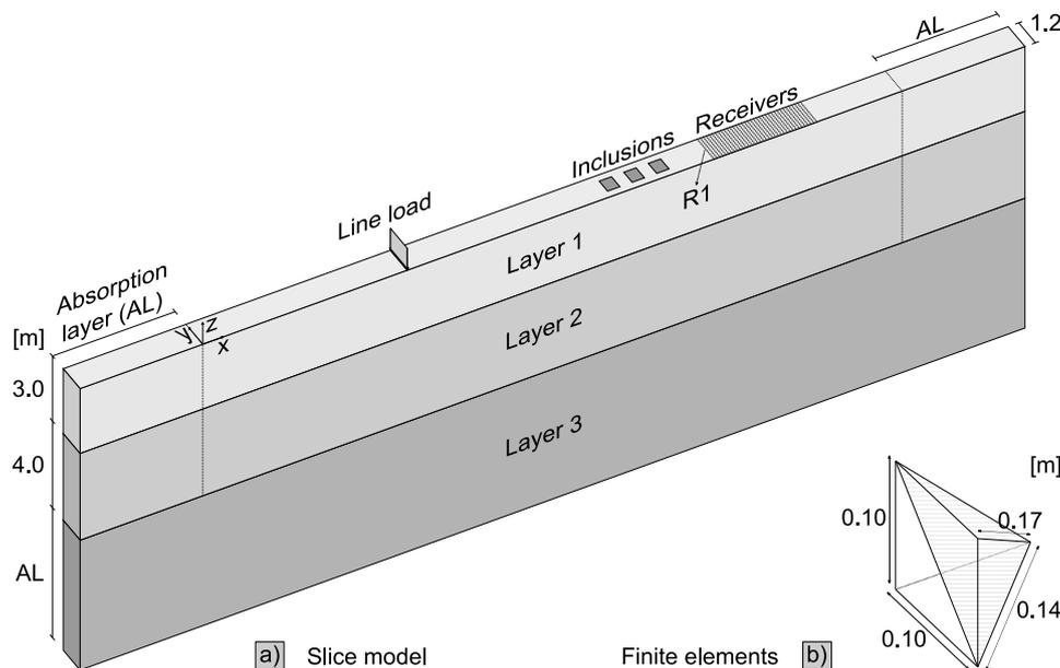
Figure 2 – a) Schematic representation of the slice model used for the wave propagation analysis and b) tetrahedral finite element example
