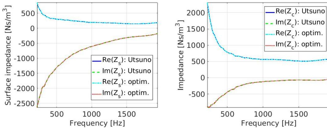
**Figure 6.** Real and imaginary part of the surface impedance (left plot) and real and imaginary part of the characteristic impedance (right plot) computed with the fitting values, taking into account both settings and considering known the low-frequency data for the dynamic mass density in comparison with respect to the Utsuno estimations.
