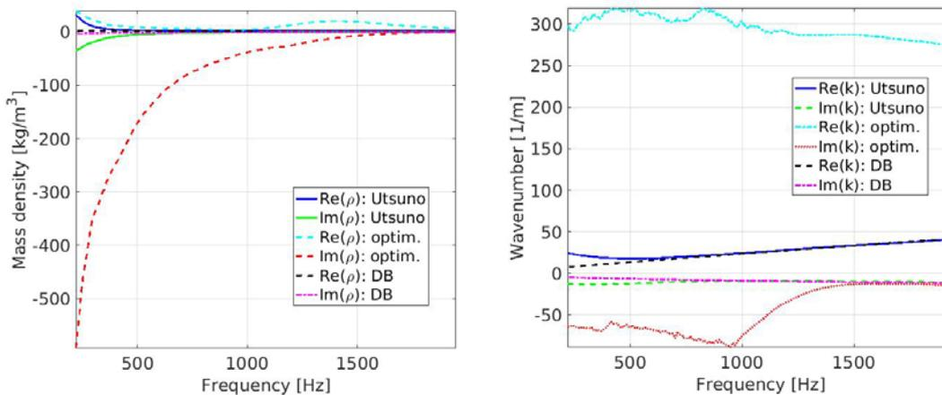
**Figure 3.** Real and imaginary part of the dynamic mass density (left plot) and real and imaginary part of the wave number (right plot) computed with the fitting values, taking into account the setting without air gap, in comparison with the Utsuno estimations and with the fitting of the Delany-Bazley model (DB).
