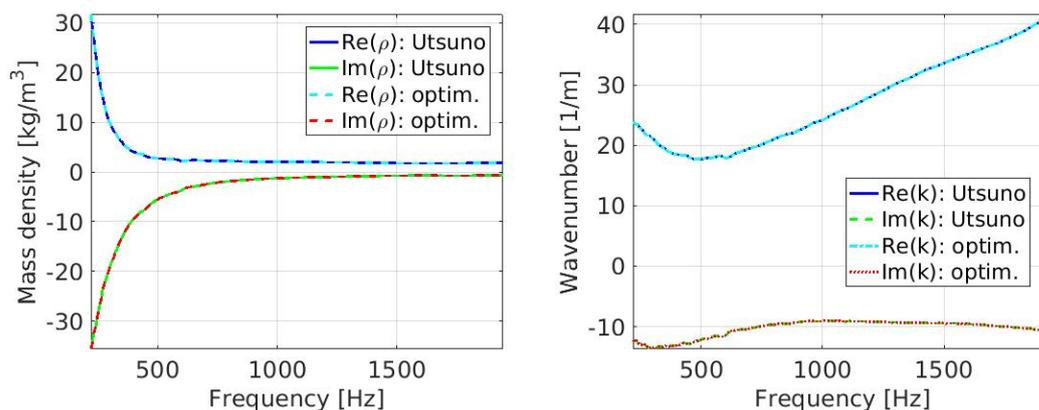
**Figure 7.** Real and imaginary part of the dynamic mass density (left plot) and real and imaginary part of the wave number (right plot) computed with the fitting values, taking into account both settings and considering known the low-frequency data for the dynamic mass density, in comparison with respect to the Utsuno estimations.
