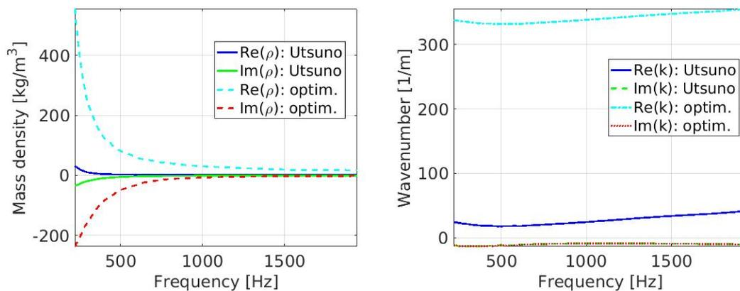
**Figure 5.** Real and imaginary part of the dynamic mass density (left plot) and real and imaginary part of the wave number (right plot) computed with the fitting values, taking into account the setting without and with air gap, in comparison with respect to the Utsuno estimations.
