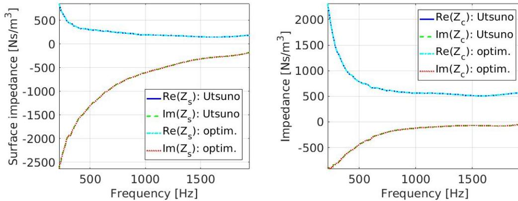
**Figure 4.** Real and imaginary part of the surface impedance (left plot) and real and imaginary part of the characteristic impedance (right plot) computed with the fitting values, taking into account the setting without and with air gap, in comparison with respect to the Utsuno estimations.
