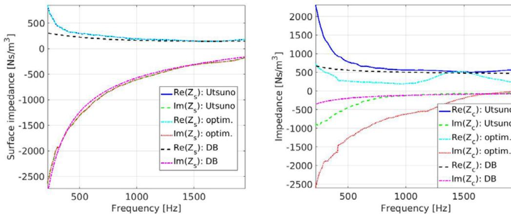
**Figure 2.** Real and imaginary part of the surface impedance (left plot) and real and imaginary part of the characteristic impedance (right plot) computed with the fitting values, taking into account the setting without air gap, in comparison with the Utsuno estimations and with the fitting of the Delany-Bazley model (DB).
