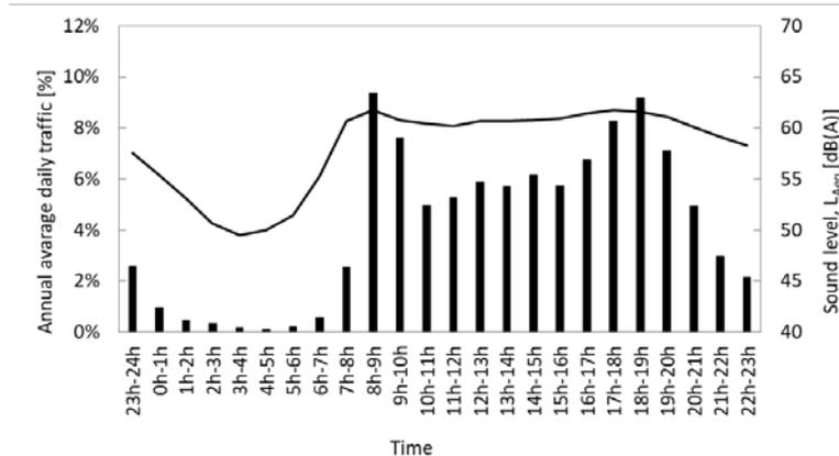
Figure 2. Relation between the traffic distribution (bars) and the temporal evolution of noise (solid line) – adapted from [14].
