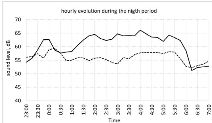
Figure 3. Comparison between the evolution of noise during the event (solid line) and without it (dashed line) – adapted from [16].
