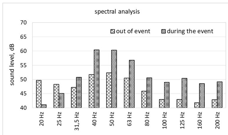
Figure 4. Comparison between the low frequency components of noise, during the event and without it – adapted from [16].
