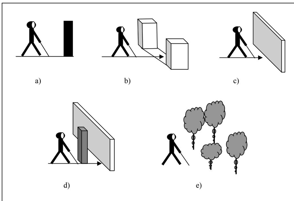
Figure 3 – Experimental scenarios: a) Single column detection; b) Two columns detection and pass through them; c) A wide wall; d) A column detection in front of a wide wall and e) Outdoor experiment.
