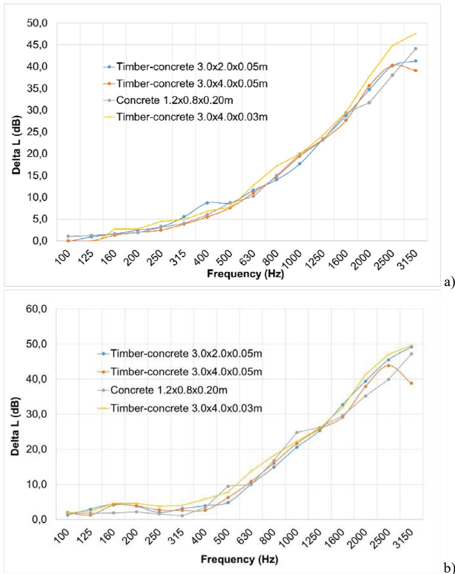
Figure 7. Impact sound reduction provided by floating floors on timber concrete floors: a) with glued cork underlayer; b) Rubber underlayer (not glued)
