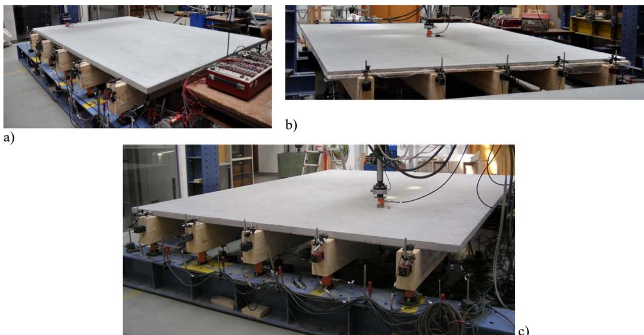
Figure 4. Images of the timber concrete slabs tested: a) 3.0x2.0x0.05(m); b) 3.0x4.0x0.03(m), c) 3.0x4.0x0.05(m)
