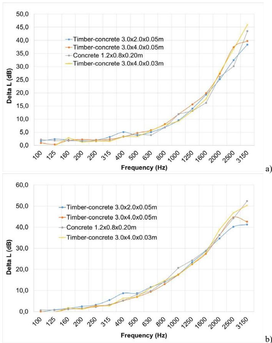
Figure 6. Impact sound reduction provided by floor coverings: a) Vinyl with flexible underlayer; b) Carpet.
