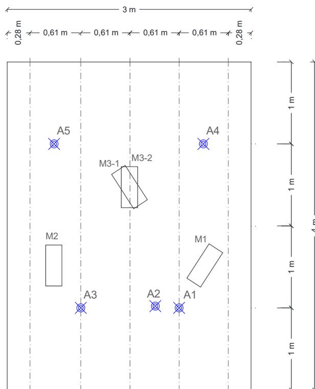
Figure 5 –Timber concrete floor with sources and measurement positions (plan).
