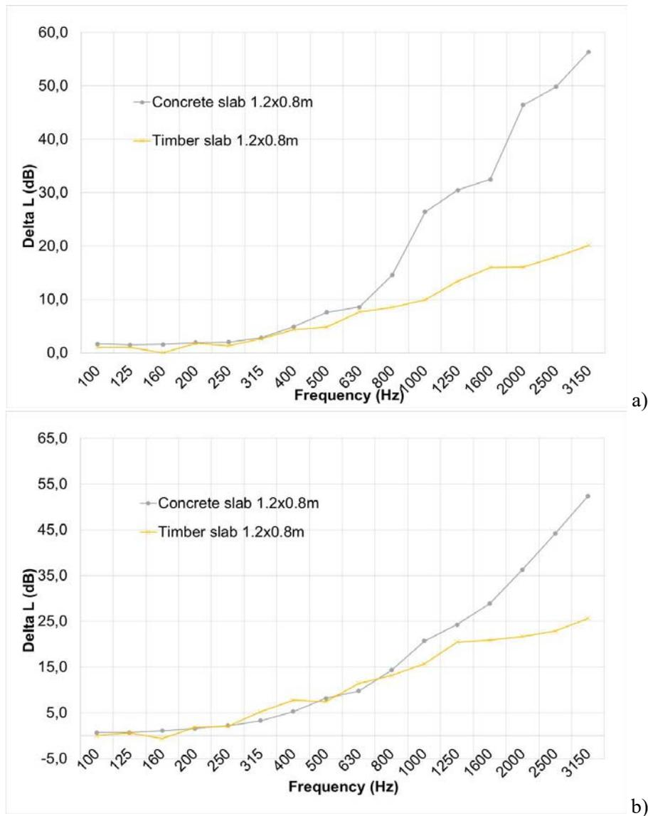
Figure 2. Impact sound reduction provided by soft floor coverings: a) Vinyl with flexible underlayer; b) Carpet.
