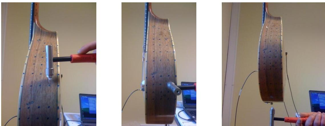
Figure 2 – Excitation at the sides at different directions and the 3 measurement position
