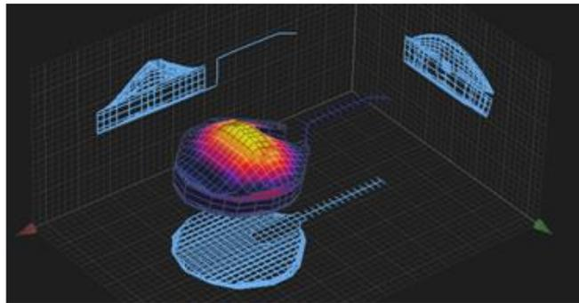
Figure 7 – Mode at 280 Hz without coupling to the air cavity mode
