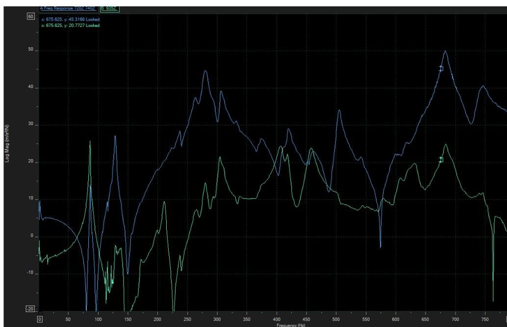
Figure 5 – 2 FRF at the soundboard measurement point: excitation at point 720 (Soundboard) and 935 (fingerboard)
