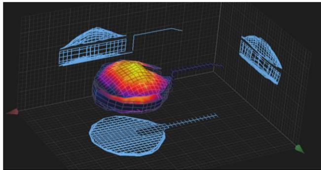
Figure 6 – Mode at 125 Hz with strong coupling with the air cavity mode
