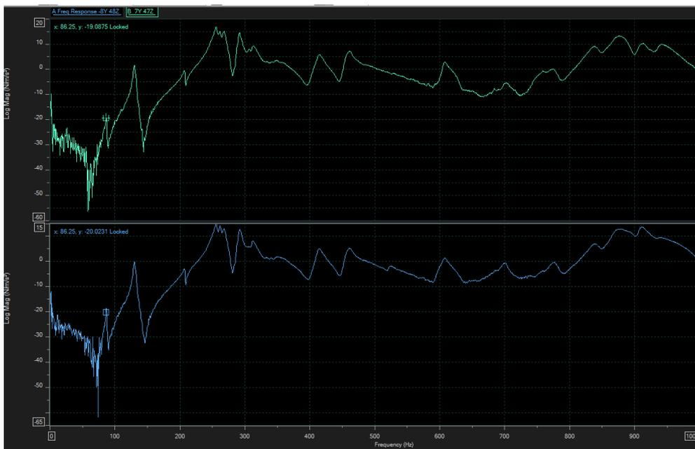
Figure 11 – FRF for 2 excitation points on the bridge (Y direction) and accelerometer beneath the 4<sup>th</sup> double string
