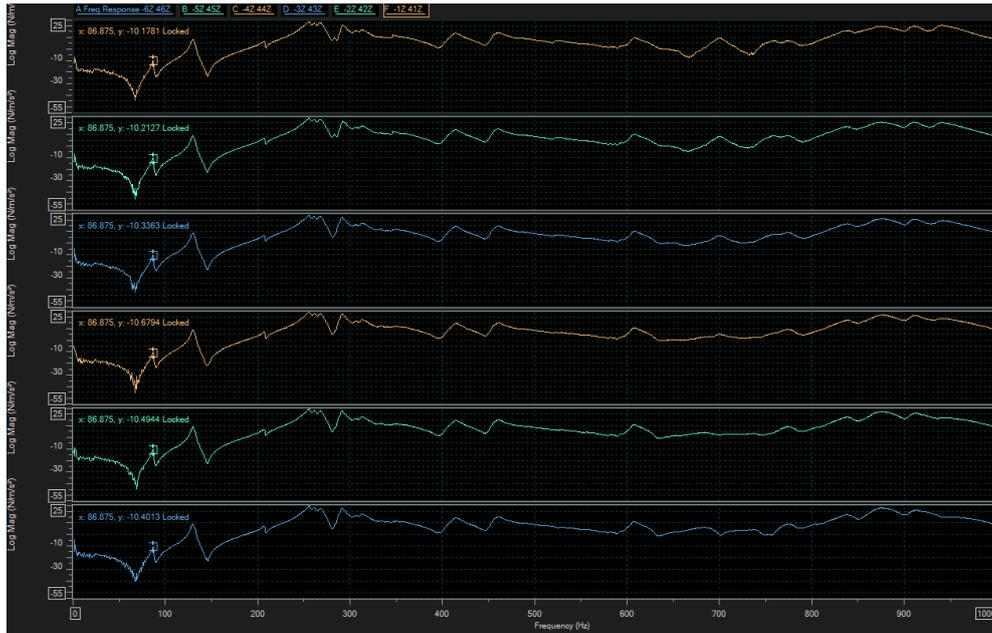
Figure 10 – FRF for 6 excitation points on the bridge and accelerometer beneath the 4<sup>th</sup> string
