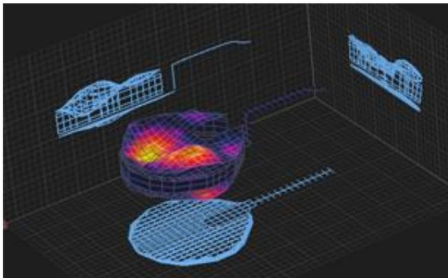
Figure 9 – Mode at 684 Hz showing the quadropole behaviour of the soundboard
