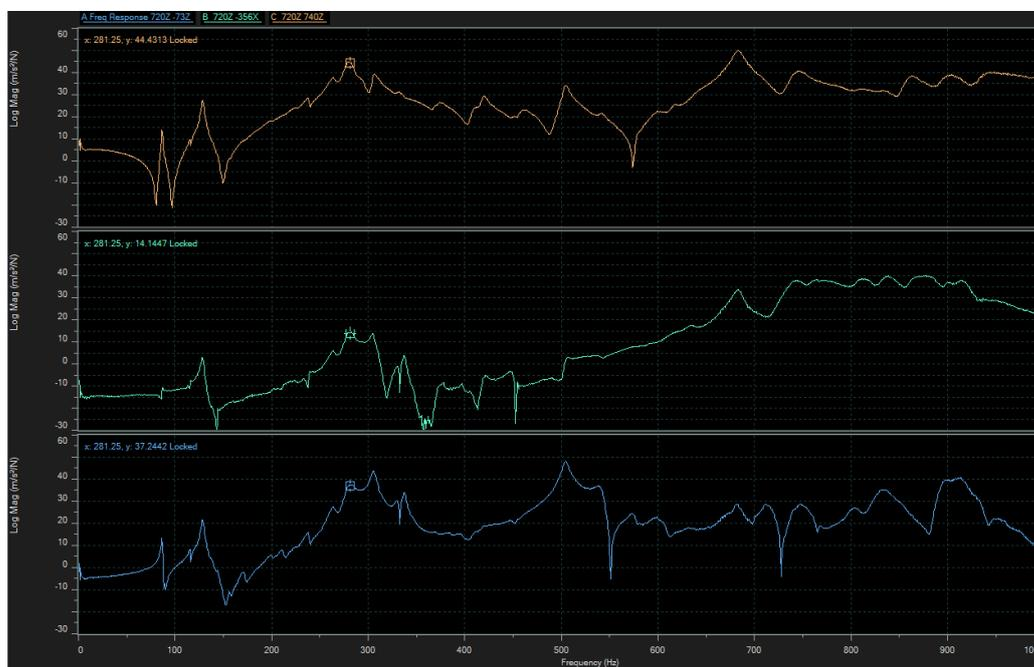
Figure 4 – 3 FRF's at each measurement point: excitation at point 720 (Soundboard)
