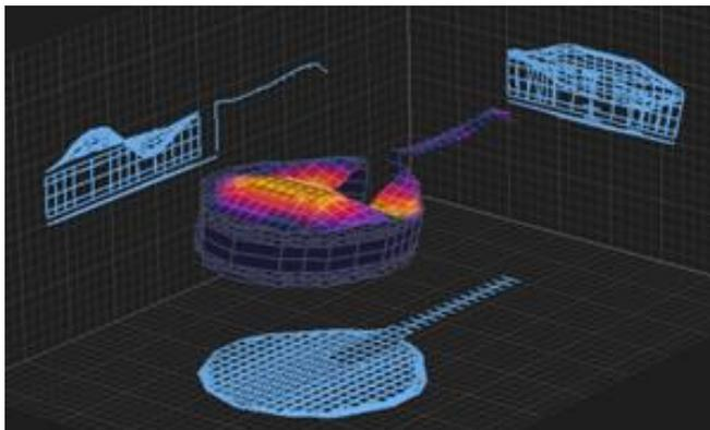
Figure 8 – Mode at 406 Hz showing the dipole behaviour of the soundboard
