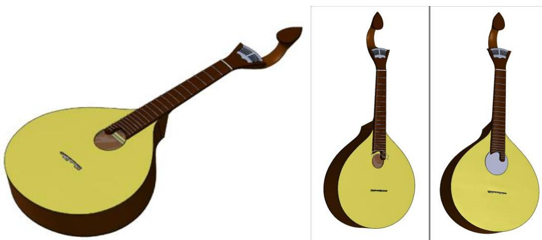
Figure 1 – Representation of the three developed 3-dimensional CAD models: at left: the original model (Model 2) [9], at the middle, the lower diameter soundhole model (Model 3) and. on the right. the higher diameter soundhole model (Model 1).
