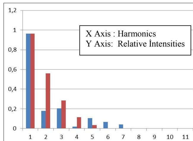
Figure 5. Red spectrum represents Cumbus. Blue spectrum represents Acoustic Guitar
