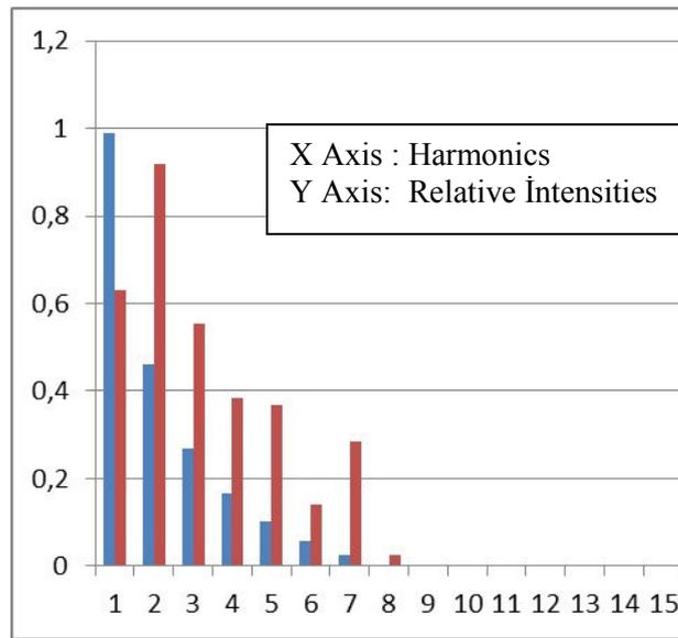
Figure 4. Red spectrum represents Electric Guitar. Blue spectrum represents Monocord's theoretical results
