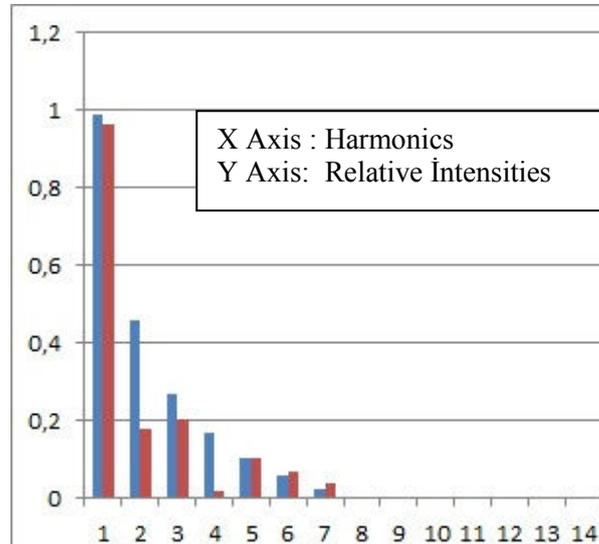
Figure 3. Red spectrum represents Acoustic Guitar Blue spectrum represents monocord's theoretical results
