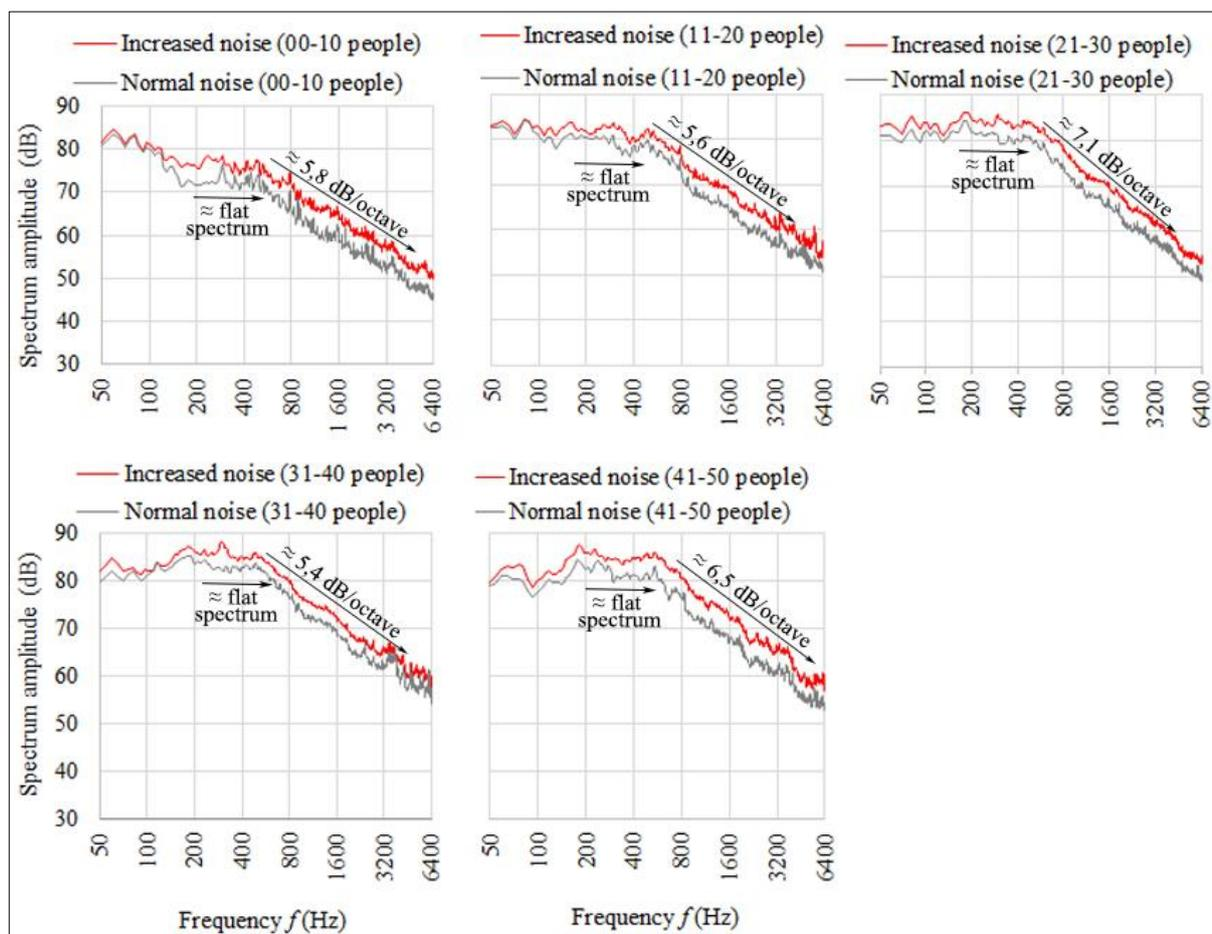
Figure 5 – Spectral analysis of steady state and noise burst fragments for different amounts of people present.
