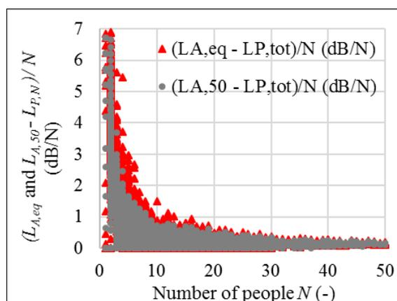
Figure 4 – Difference  $L_{A,eq}$  (dB) -  $L_{P,tot}$  (dB) (red triangles) and  $L_{A,50}$  (dB) -  $L_{P,tot}$  (dB) (black dots) versus number of people present.
