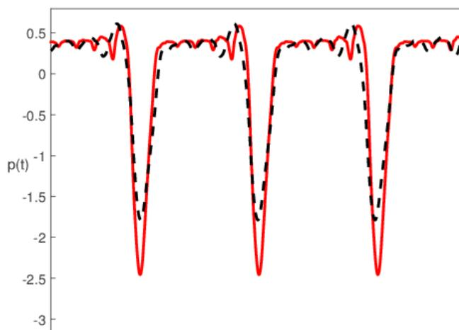
Figure 3: Two waveforms for the mouthpiece pressure calculated with the minimum model. The total length is the same for the two cases:  $L=1.3\text{m}$ . Solid line:  $x_1 = 0.2\text{m}$ . Dotted line:  $x_1 = 0.3\text{m}$ . The pressure  $p(t)$  is reduced by the static closure pressure.
