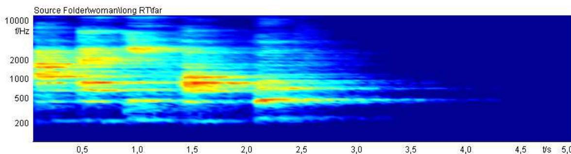
Figure 4 – Spectrograms of female voice in a classroom with long reverberation time at the position of 2 m from the virtual teacher
