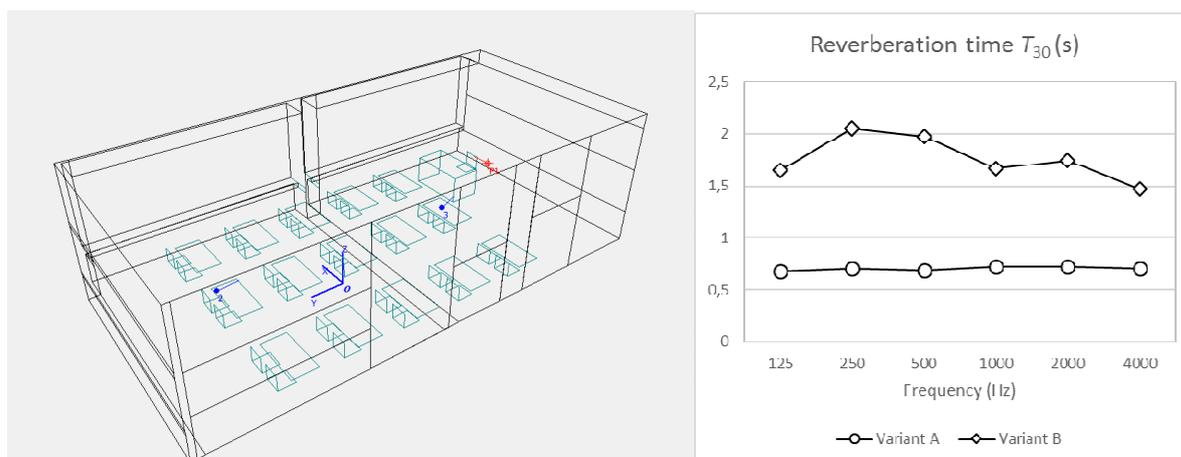
Figure 1 – Virtual model of classroom used for simulations. Two different reverberation time values  $T_{30}$  were used.
