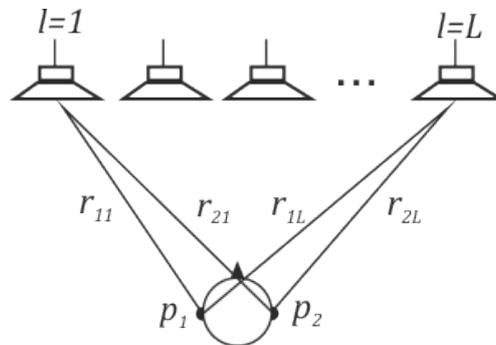
Figure 1: Geometry of the loudspeaker array used to control the acoustic pressure at the listener's ears.
