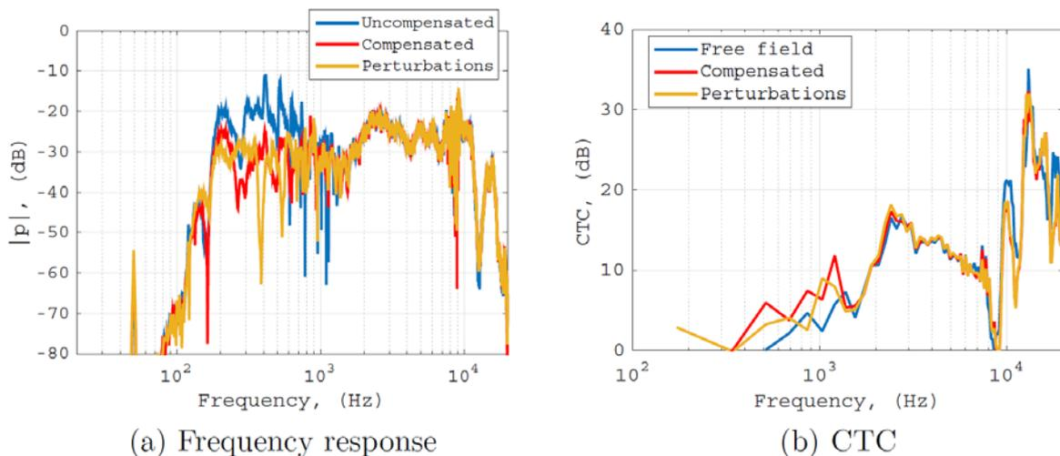
Figure 6: Measured frequency response and cross-talk cancellation performance in the setup of Fig. 5 for free-field filters (Uncompensated), compensation filters (Compensated) and compensated filters with modified wall distances to introduce errors (Perturbations).
