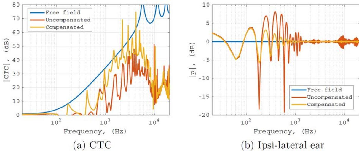
Figure 3: Cross talk cancellation and frequency responses under the effect of lateral reflections (“Uncompensated”) and when these are compensated (“Compensated”) compared with the free-field performance.
