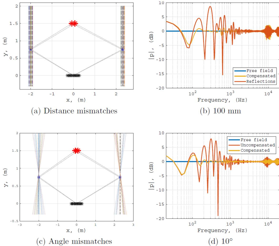
Figure 4: Average performance of the array for errors with a standard deviation of 10 cm (top plots) and 10 degrees (left plots).
