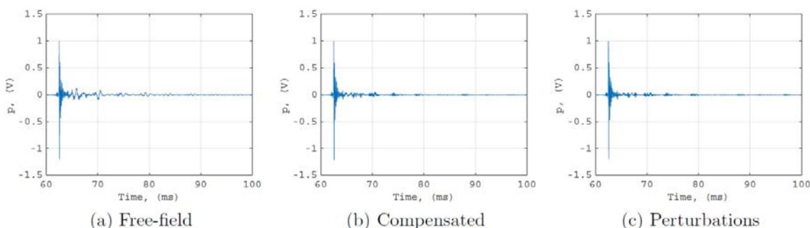
Figure 7: Measured impulse responses in the setup of Fig. 5 for free-field filters (Uncompensated), compensation filters (Compensated) and compensated filters with modified wall distances to introduce errors (Perturbations).
