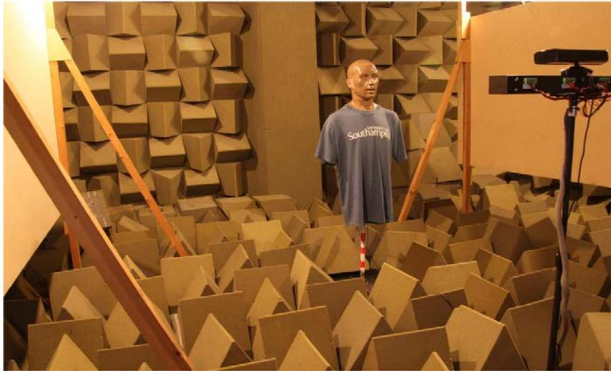
Figure 5: Setup used for the practical measurements.
