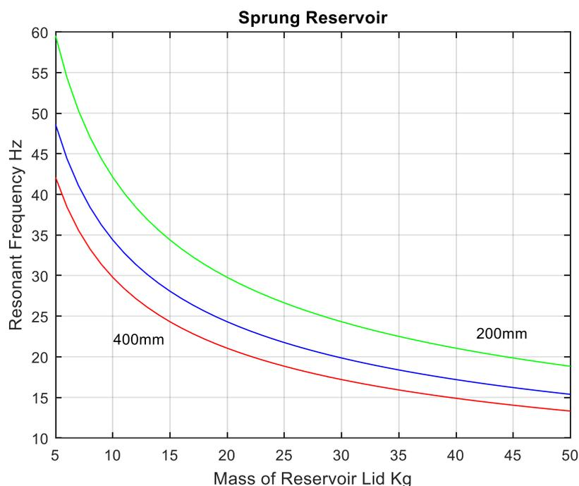
Figure 8 – Resonant Frequency for Sprung Reservoir
