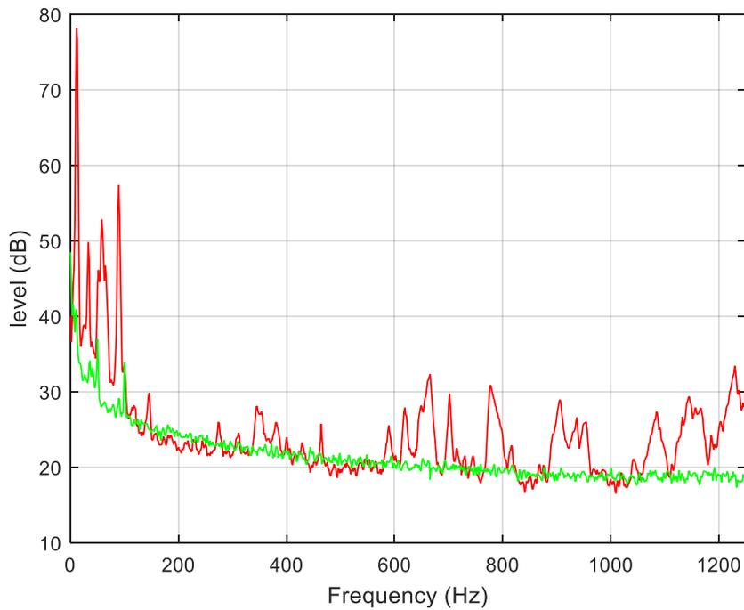
Figure 5 – Reservoir Vibrations for Electrically Blown (red) and Hand Blown (green)
