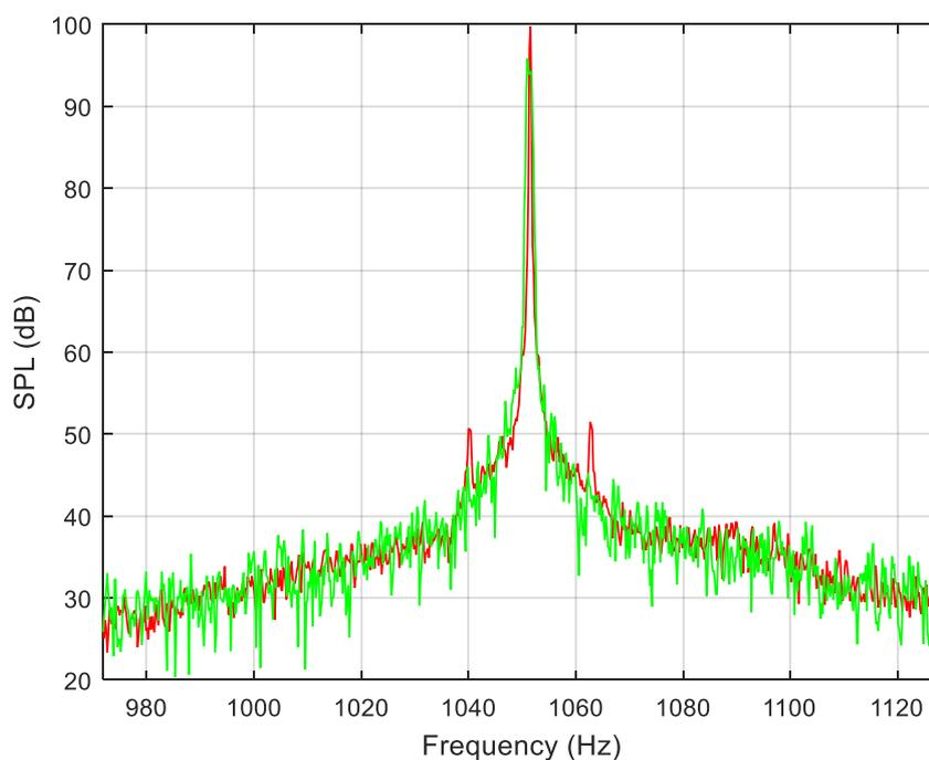
Figure 4 – Expanded Fundamental for Electric Blown (red) and Hand Blown (green)
