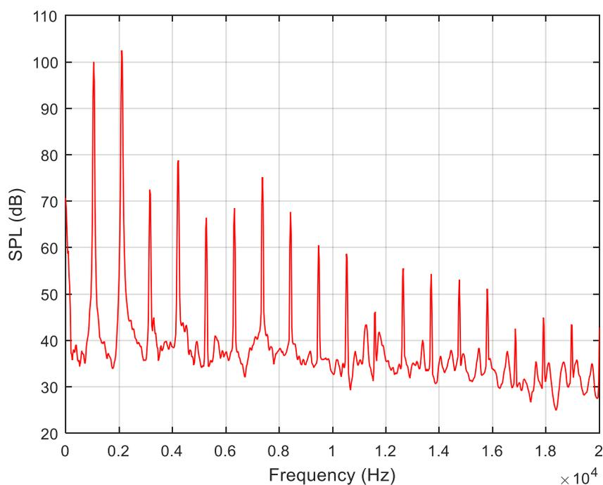
Figure 3 – Frequency Spectrum of a treble c pipe
