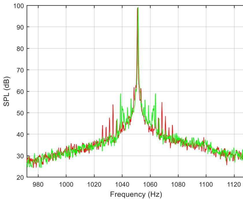
Figure 6 – Weighted (green) and Sprung (red) Reservoir Tremulant modulation
