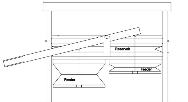
Figure 1 – Double Rise Reservoir and Feeders
