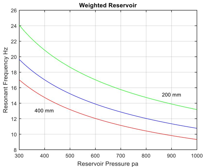
Figure 7 – Resonant Frequency for Weighted Reservoir
