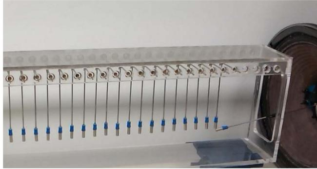
Fig. (1) The experimental setup shows that the pendulums are totally "hanging" by the repulsion force between two disc magnets.
