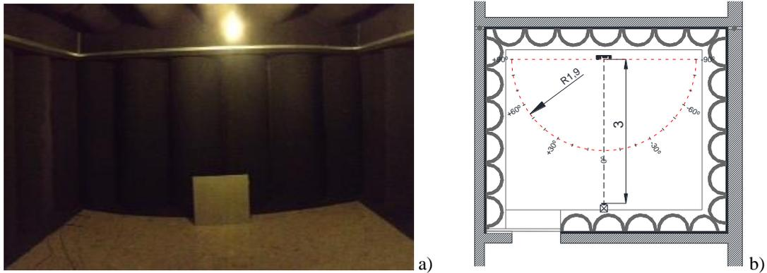
Figure 1 – Simplified semi-anechoic room: a) image of the interior, looking at the specimen's location; b) layout configuration for diffusion coefficient evaluation.
