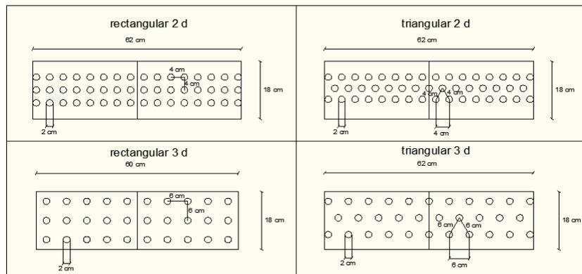
Figure 2 – Schematic representation of some of the sonic crystal structures tested.
