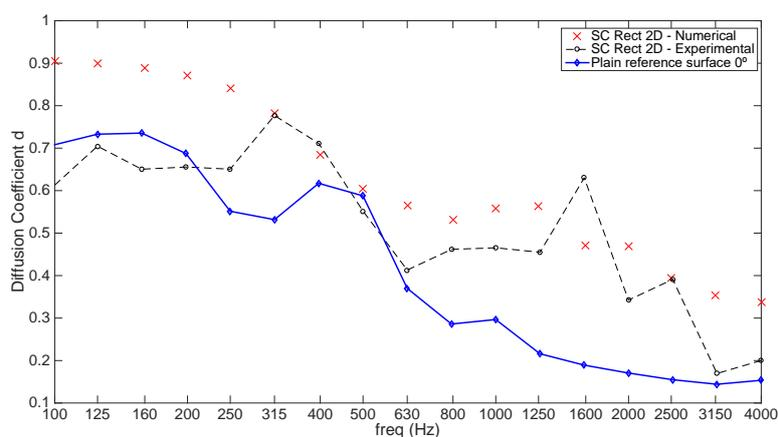
Figure 4 –Diffusion coefficient for a sonic crystal with rectangular lattice: comparison between measured data and computed results.
