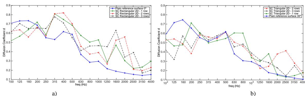
Figure 3 – Diffusion coefficient of periodic structures measured in semi-anechoic conditions: a) rectangular lattice (2D) with  $0^\circ$  sound incidence; b) triangular lattice (2D) with  $35^\circ$  sound incidence.
