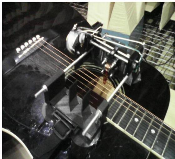
Figure 2 – Robots plucking module.
