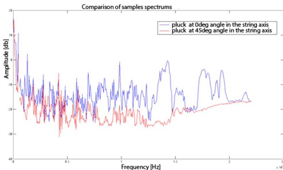
Figure 5 – Two samples that had different pluck angle, set on one graph for comparison purposes
