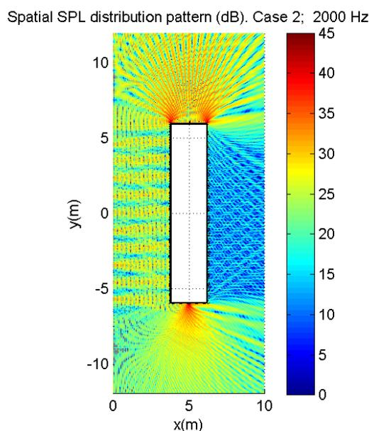
Figure 4 – Effect of a reflective wall on the sound pressure field. Case 2, 2000Hz.
