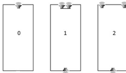
Figure 1 – Three cases of AVAS configurations
