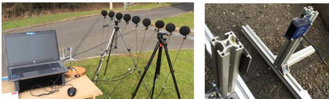
Figure 2– A. ULA Microphone array and analyzer used during the tests. B. Photocell used to determine the location of the vehicle.
