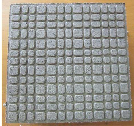
Figure 4 – Paving stone with an acoustically optimized macrotexture.
