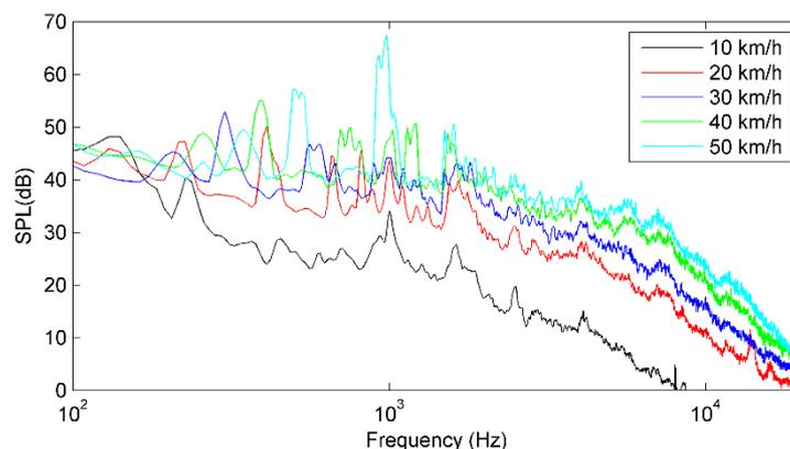
Figure 5. Evolution of the frequency spectrum with the speed for an electric moped.
