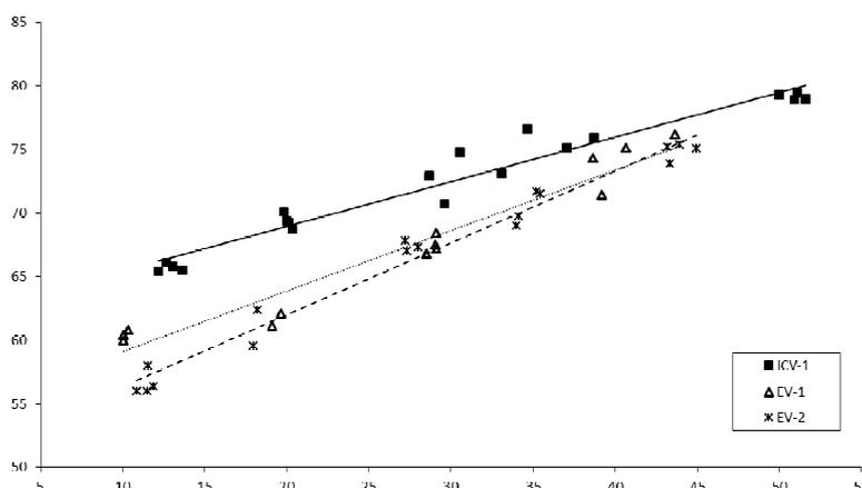
Figure 3. Maximum Sound Pressure Level emitted by mopeds with power smaller than 7 kw at different speeds.
