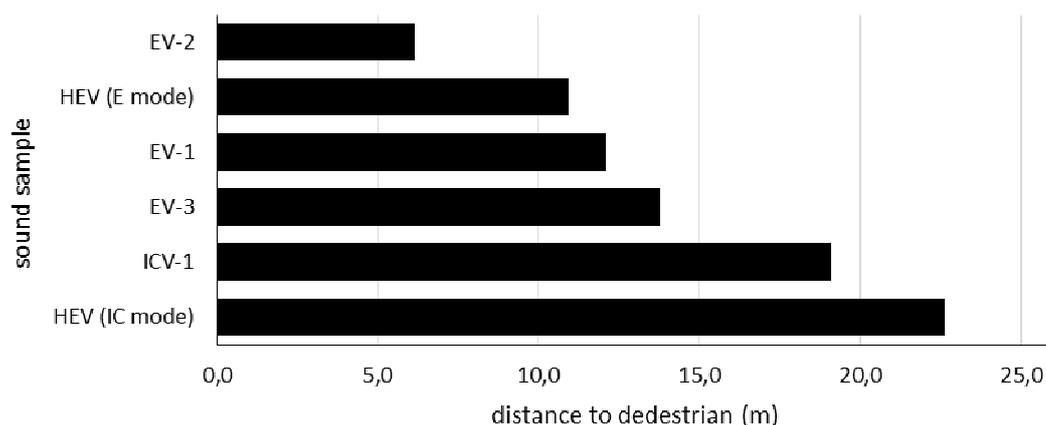
Figure 6. Distance to pedestrian for different two-wheeled vehicles.
