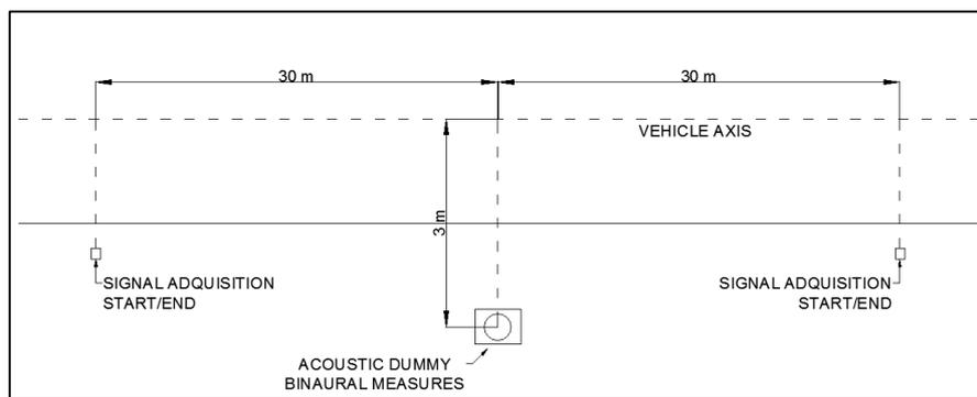
Figure 2. Pass-by test configuration for sound samples acquisition.
