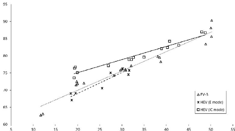
Figure 4. Maximum Sound Pressure Level emitted by mopeds with power greater than 7 kw at different speeds.
