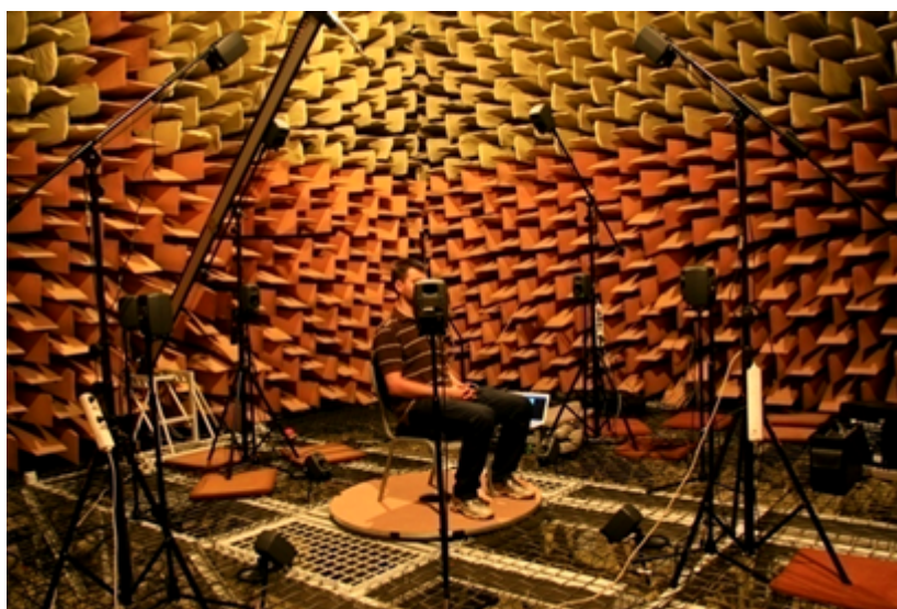
Figure 1 – The position of listening tests with a multi-channel system installed in the anechoic chamber.
