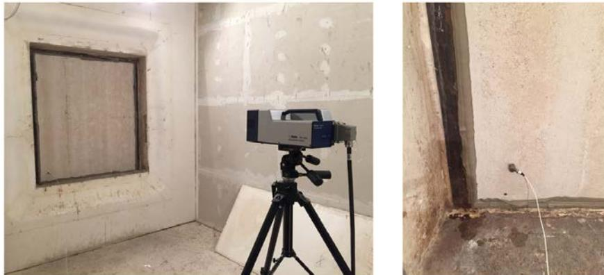
Figure 3 – Construction mounted by putty into the window measurement frame and reference accelerometer position for the laser vibrometry measurements
