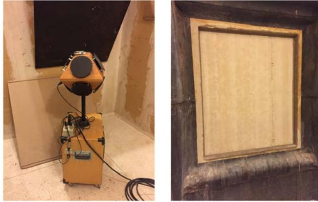
Figure 4 – Loudspeaker for airborne excitation and backside of the construction mounted by putty into the window measurement frame
