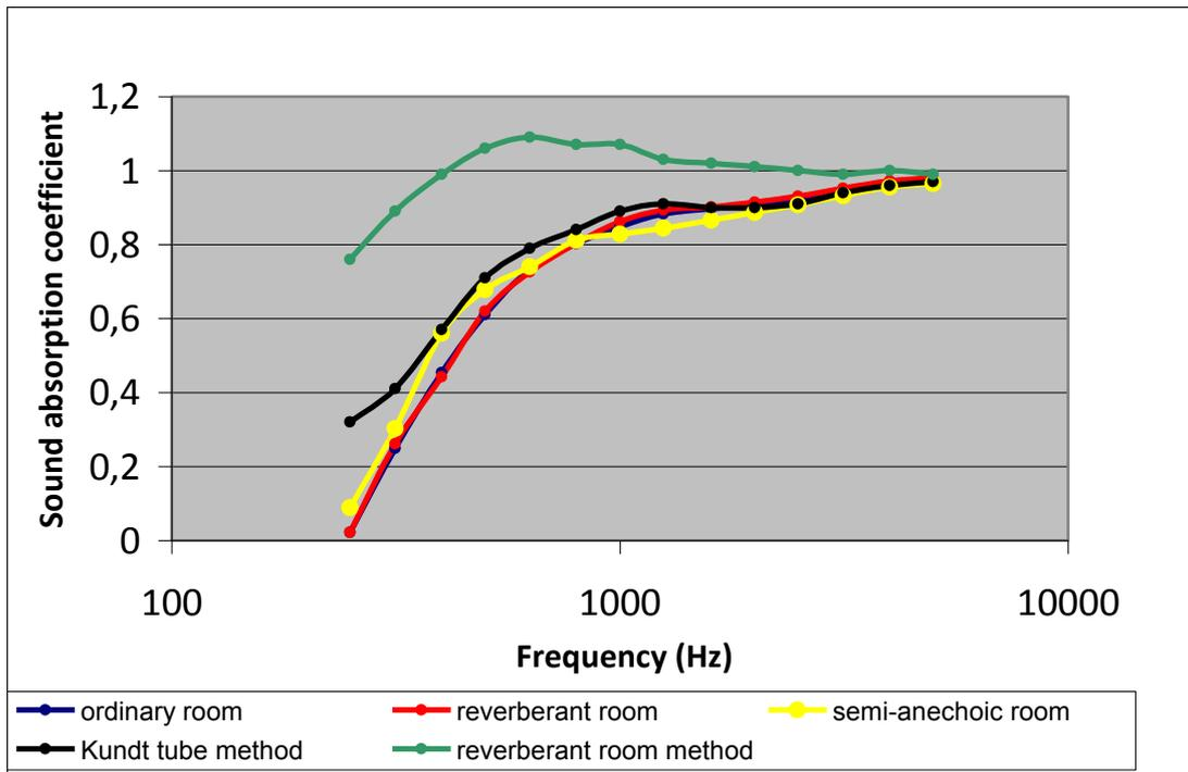
**Figure 4.** Sound absorption coefficient measured for the rock wool sample by means three different techniques. The sound absorption coefficient measured in different environments by the PU probe has been included in the figure.
