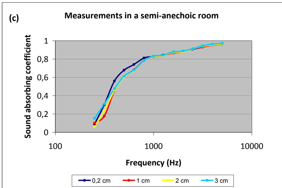
**Figure 2.** Sound absorption coefficient measurement at three different environments: (a) an ordinary room, (b) a reverberant room and (c) a semi-anechoic room. The sound absorption coefficient is plotted for four distances PU probe-sample surface.
