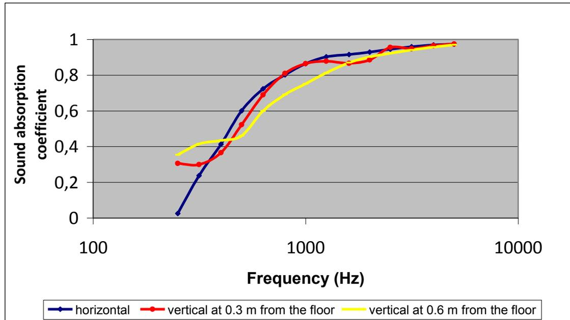
**Figure 3.** Sound absorption coefficient measurement in the reverberant room with the sample placed in horizontal on a rigid surface and in vertical position. In the last case the PU probe has been placed at two different distances from the floor. The distance PU probe-sample surface was 1.5 cm.
