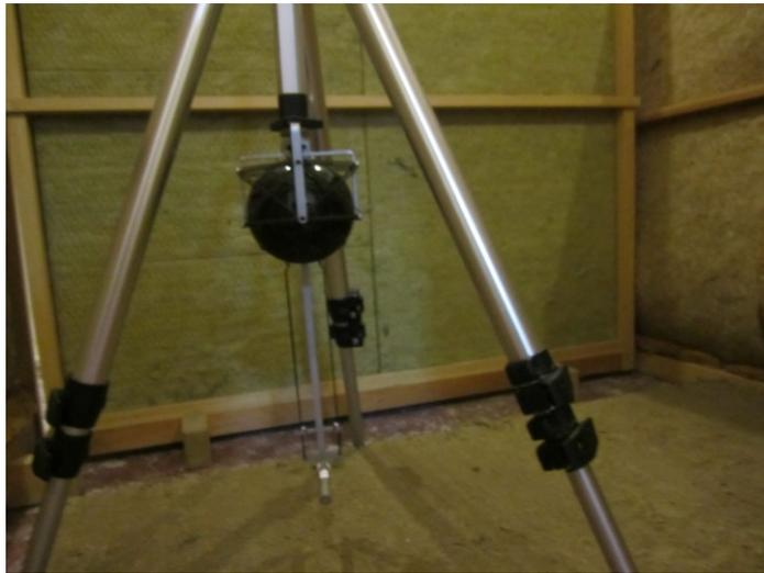
**Figure 1.** Picture of the assembly used for the PU probe for the measurements.
