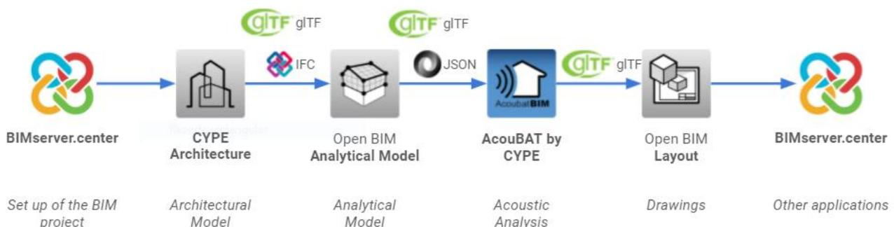
Figure 1 – Acoustic workflow diagram.
