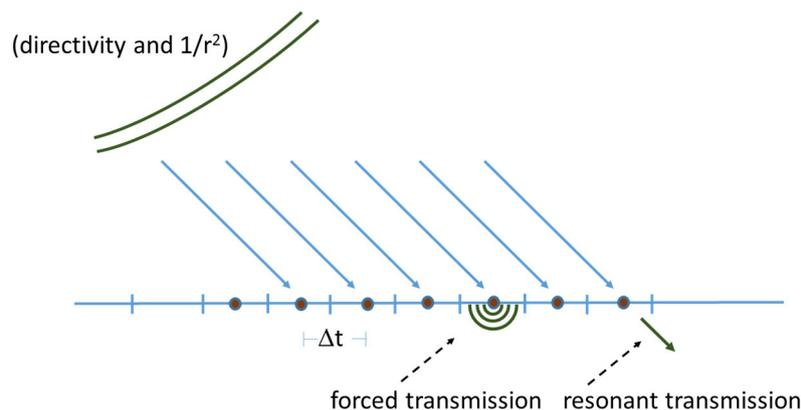
Figure 2 – Excitation of a grid of patches building façade with oblique incidence and radiation from secondary sources
