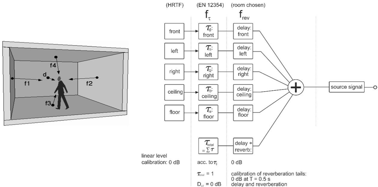
Figure 1 – Left: Geometric situation. Right: Flow chart of airborne sound auralization (after [11]).
