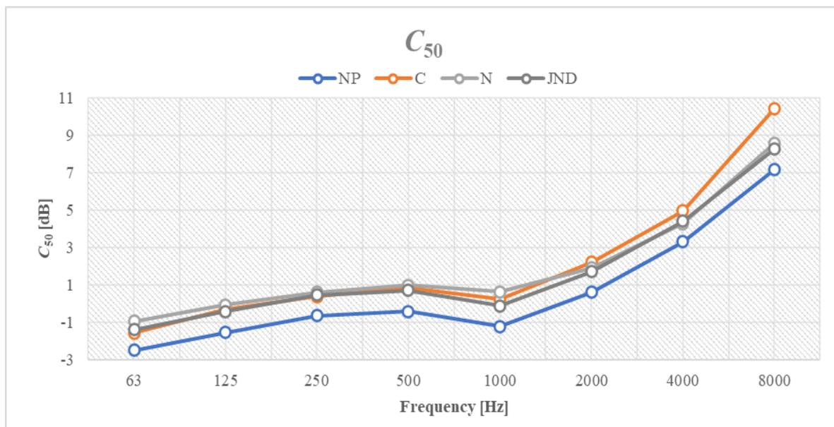
Figure 5 –  $C_{50}$  of the model without the pulpit, with the pulpit in the nave and with the pulpit in the crossing
