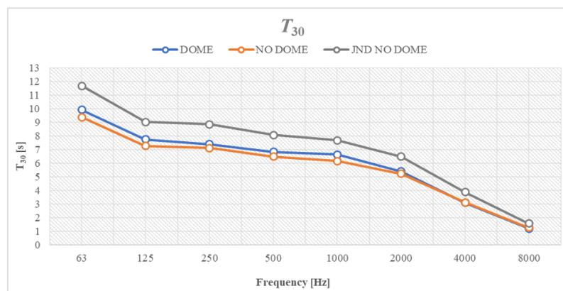
Figure 2 –  $T_{30}$  of the model with or without dome
