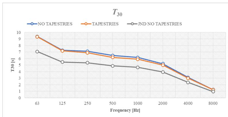
Figure 3 –  $T_{30}$  of the model with or without tapestries
