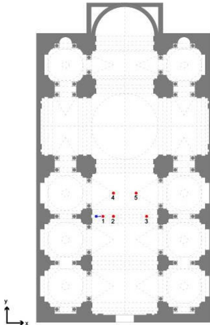
Figure 6 – Positions of the five receivers in the nave
