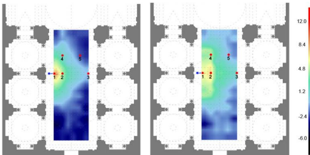
Figure 8 –  $C_{50}$  [dB] of the five receivers of the model without (left) and with the pulpit in the nave (right)
