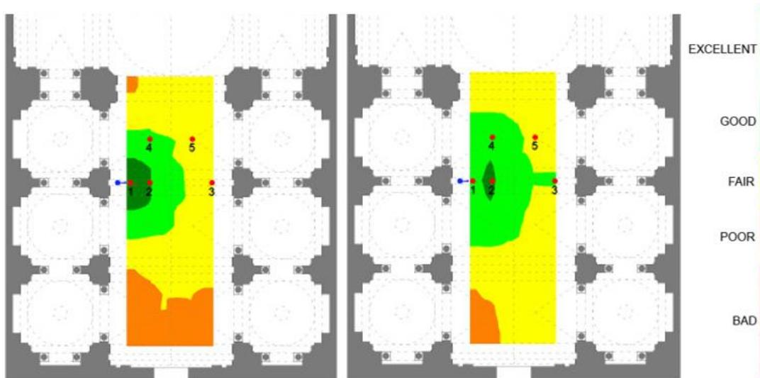
Figure 9 – STI of the five receivers of the model the without (left) and with the pulpit in the nave (right)
