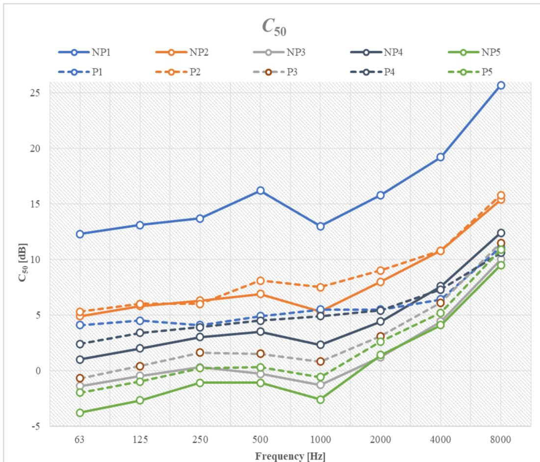
Figure 7 –  $C_{50}$  of the five receivers of the model without and with the pulpit in the nave
