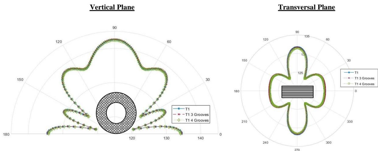
Figure 7 - Sound pressure level for Tyre 1 with different surfaces at 1000 Hz polar charts.
