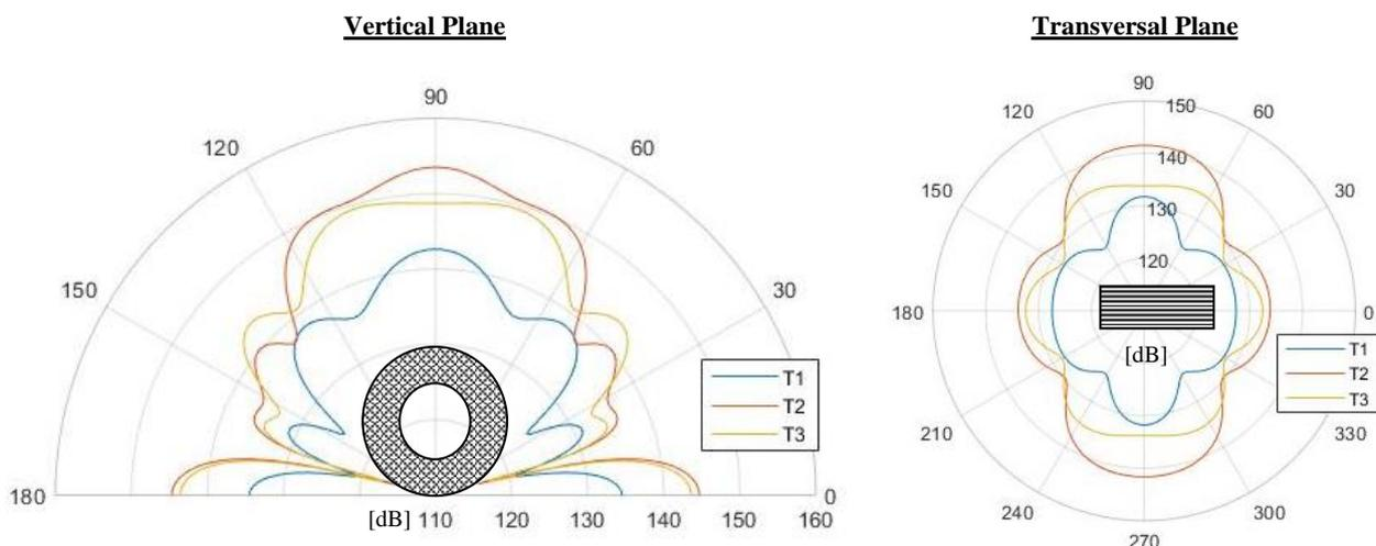
Figure 5 – Sound pressure level for different tyres at 1000 Hz polar charts.
