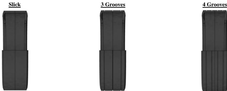
Figure 6 – Tyre 1 geometries with different surfaces.
