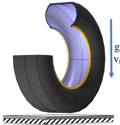
Figure 2 - Modelling of the FEM analysis with a three-quarter view of the tyre.
