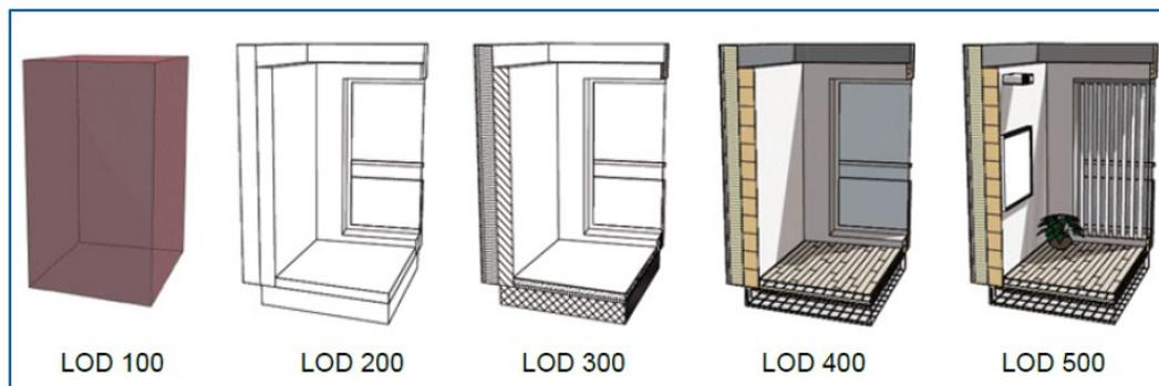
Figure 4 – Example of different Level of Detail in the IFC data model [8]
