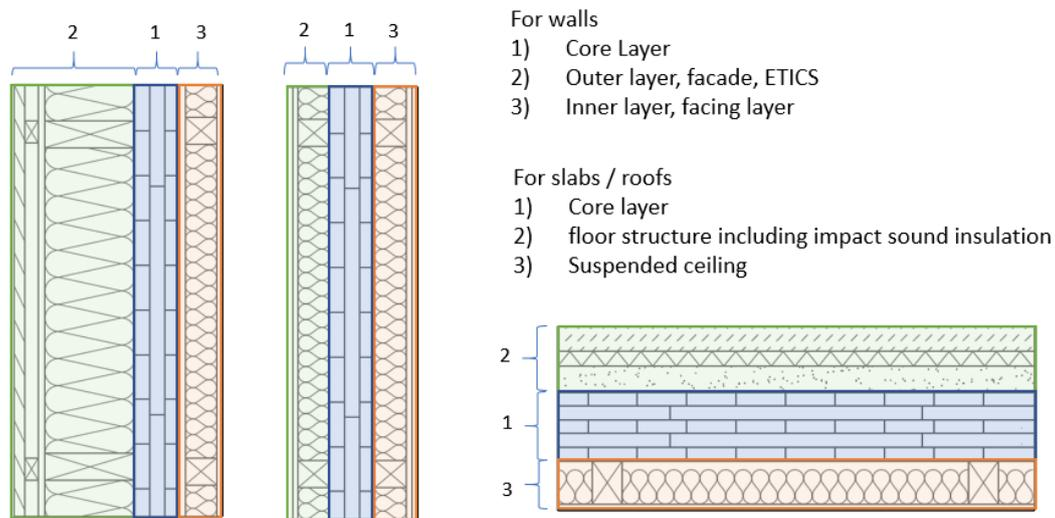
Figure 6 – Example of the inner layer, core layer and outer layer for different elements
