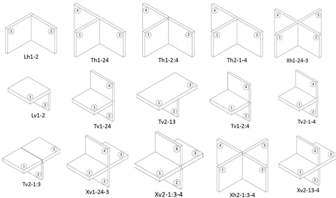
Figure 5 – Types of junctions between building elements relevant for sound insulation according to [9]
