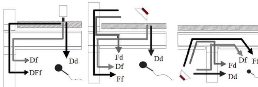
Figure 3 – Sound transmission paths with the paths  $Ff$ ,  $Df$ ,  $Fd$  and  $DFf$  for the impact sound transmission of a ceiling (left), sound insulation of a ceiling (middle) and sound insulation of a wall (right) [6]
