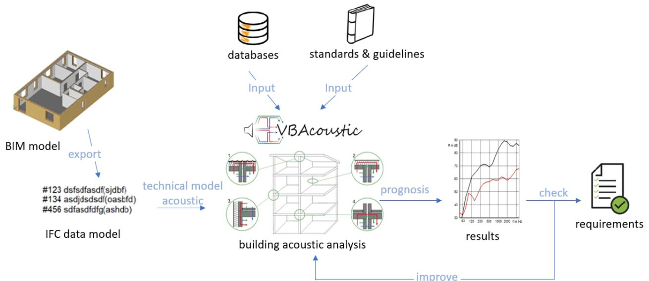
Figure 2 – Overview of the planning process for building acoustics using VBAcoustic for the prediction of the apparent sound insulation and the apparent normalized impact sound level
