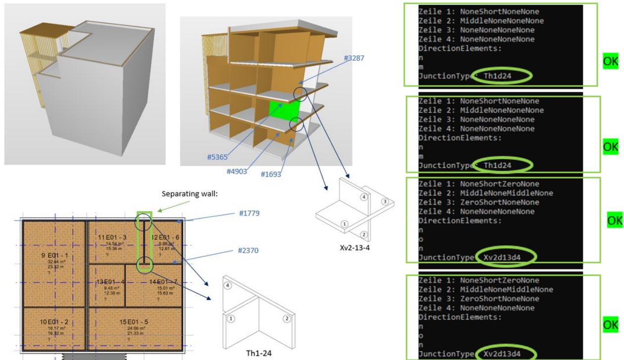
Figure 8 – Use case building with *ifcWall* as separating element and different flanking elements. The results for the junction types determined are displayed on the right-hand side in the console output.
