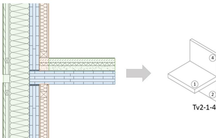
Figure 7 – Example of a junction detail for cross laminated timber elements with a slab and two walls as flanking elements: the core layer determines the junction type Tv2-1-4
