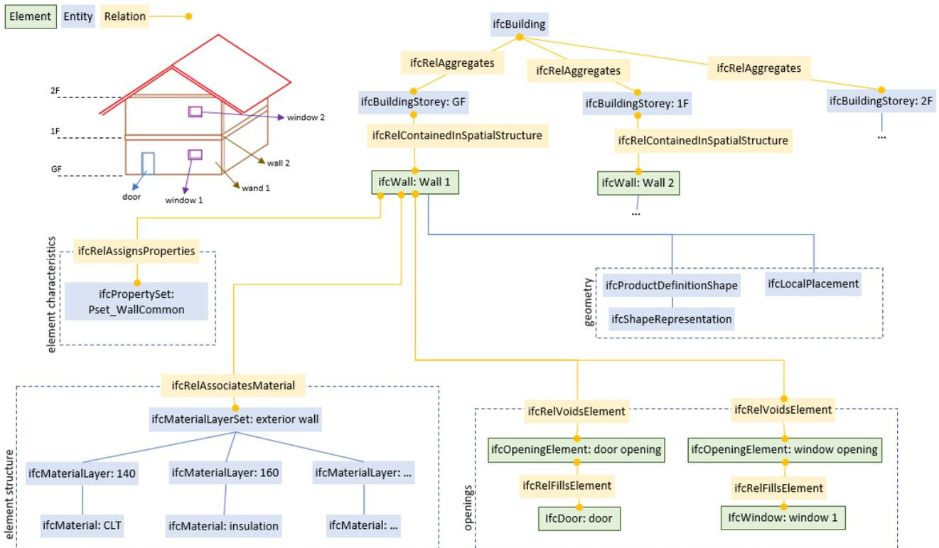
Figure 1– Schematic structure of an IFC file (shortened and simplified)
