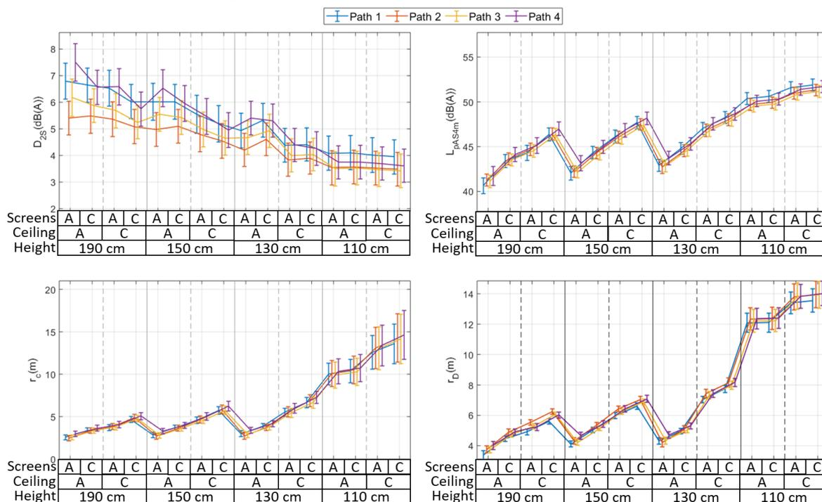
Figure 4 – Mean values and 95% confidence interval of the SNQs of ISO 3382-3 for the four measurement paths in each of the 16 acoustic configurations
