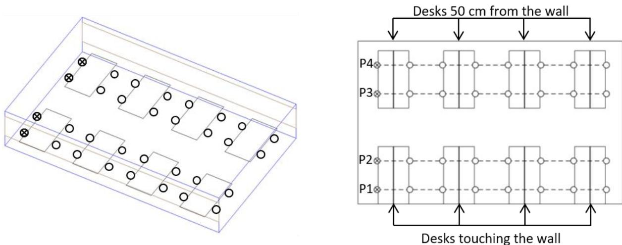
Figure 2 – Layout of the simulated office with 32 workstations and the four measurement paths (dashed lines) numbered from P1 to P4. (Circles: microphones, Crossed circles: sources)
