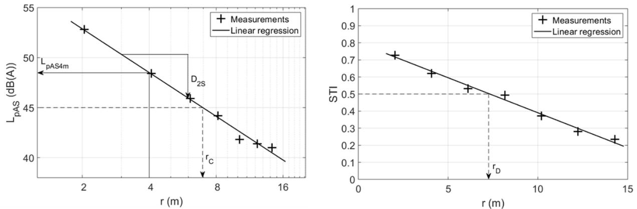
Figure 1 – Evaluation of the SNQs according to ISO 3382-3 standard.
