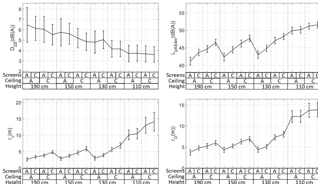
Figure 5 – Mean values and 95% confidence interval for each of the 16 acoustic configurations considering that the office is described by a unique value for each SNQ.
