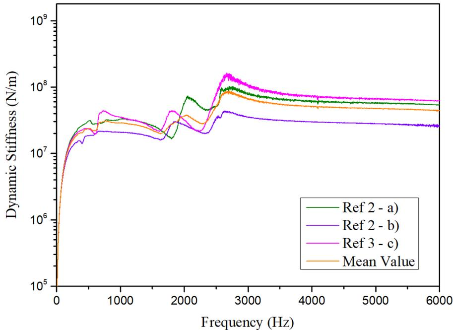
**Figure 2** - Stiffness spectrum of the samples of reference two and mean stiffness spectrum.
