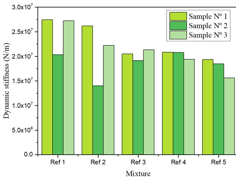
**Figure 4** - Dynamic stiffness values obtained in the individual samples at 400 Hz.
