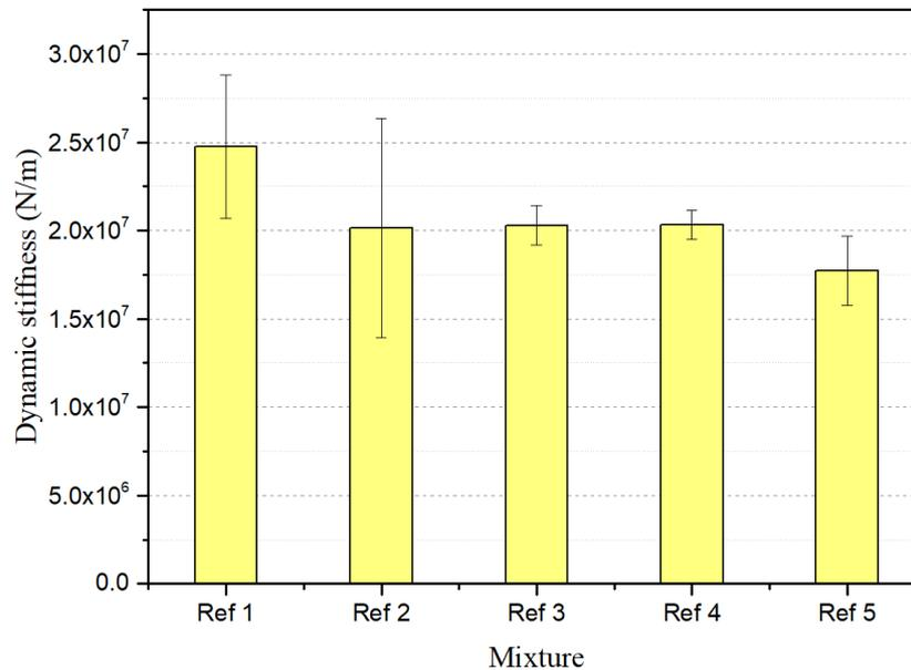
**Figure 5** - Graphic of mean values of dynamic stiffness and standard deviation for the reference series at 400 Hz.
