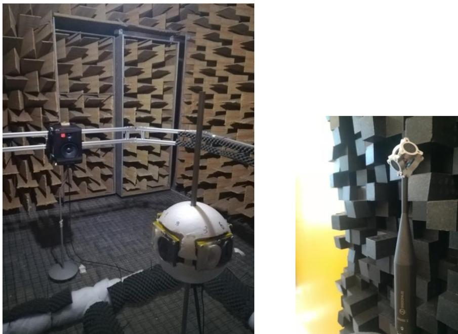
Figure 8 – Microphone systems, OctoEar and AMBII used to capture 3D sound in an anechoic chamber.
