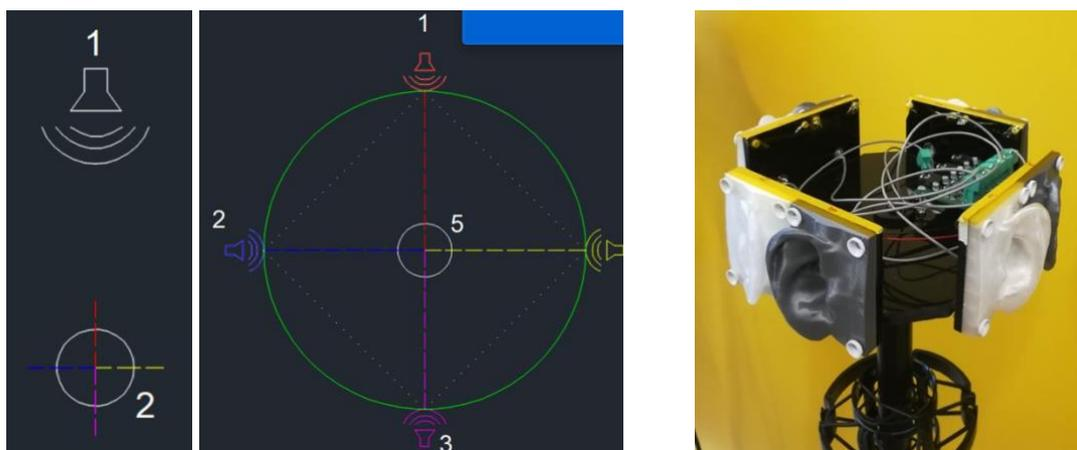
Figure 3 - System basic scheme and a photograph of the OctoEar, apparatus with 4 pairs of ears.
