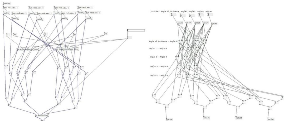
Figure 10 - PureData patches used for live recordings (left) and the sub-patch for weighting values (right).
