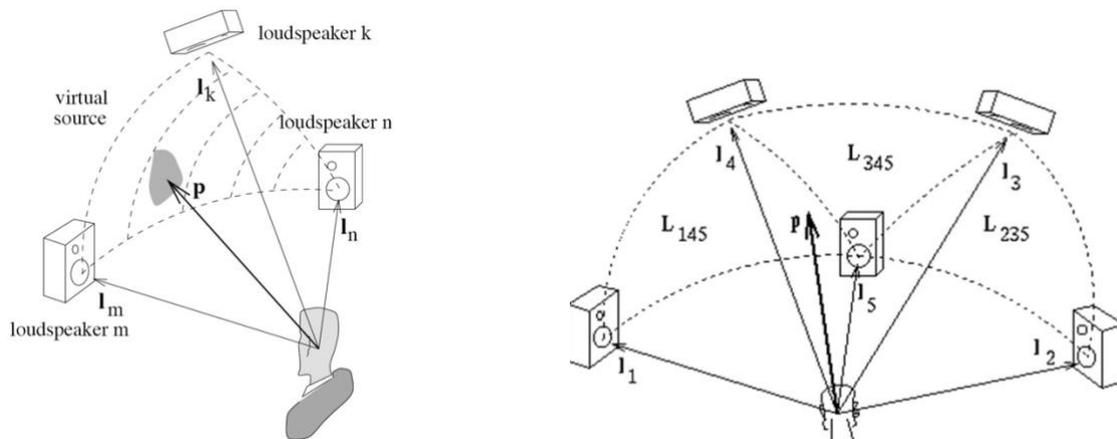
Figure 2 – Vector-based amplitude panning (VBAP) technique.
