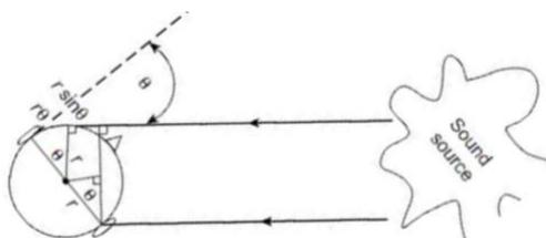
Figure 1 – Basic scheme for the Interaural Time Difference (ITD) cue.
