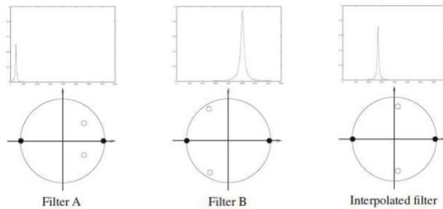
Figure 3 – Pole-zero diagrams and spectral interpolated filter.
