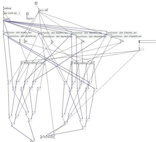
Figure 9 – PureData patch used to implement the HRTF filtering depending on the desired angle.
