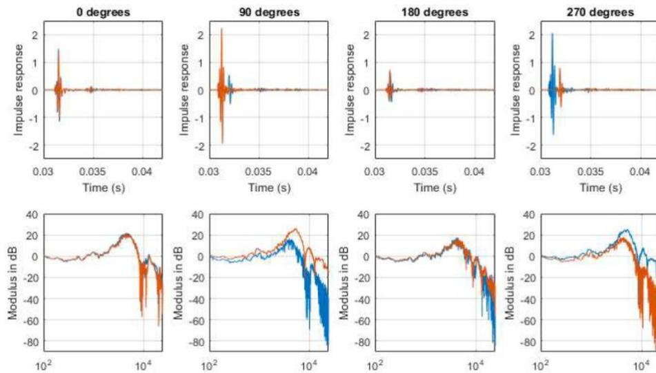
Figure 4 – HRTF for the 4 pairs of ears measured with the OctoEar apparatus.
