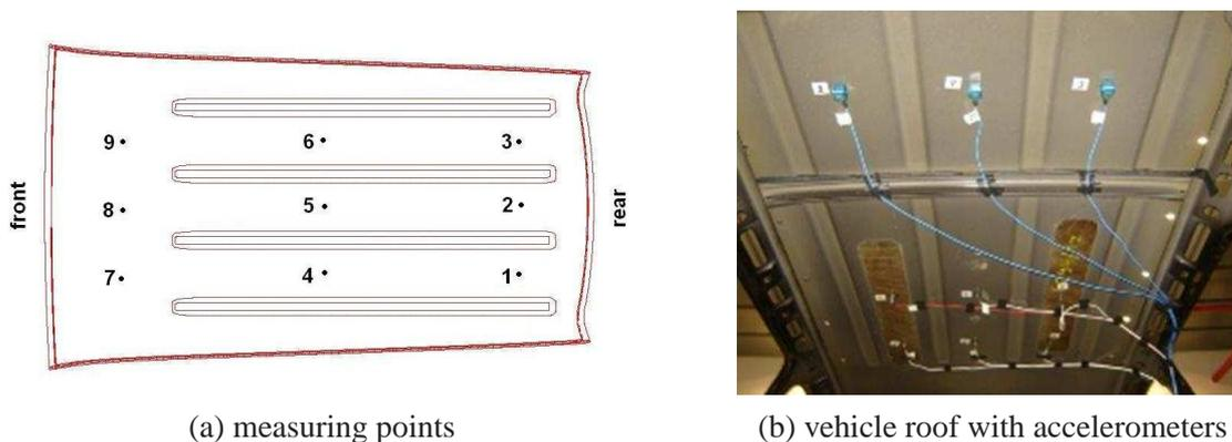
**Figure 2:** Mesh of measuring points in the vehicle roof.
