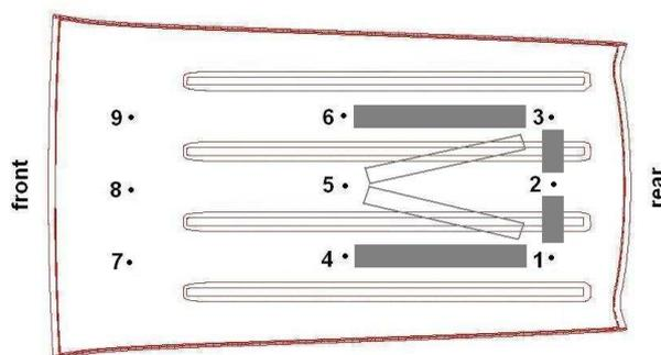
**Figure 6:** Areas that have higher influence on the critical FRFs in the frequency range of 60 to 80 Hz.
