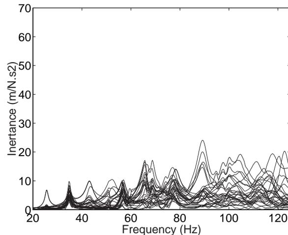
**Figure 8:** FRFs of the vehicle roof with deadeners at positions defined with help of the embedded sensitivity method.
