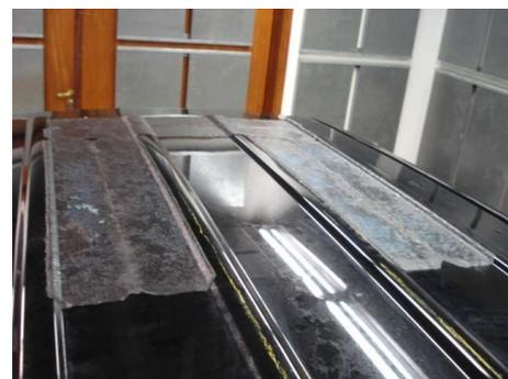
**Figure 7:** Deadeners fixed on the vehicle roof (modified structure).
