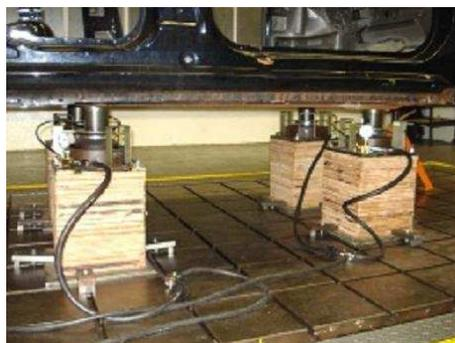
**Figure 3:** Vehicle body supported by pneumatic benches.
