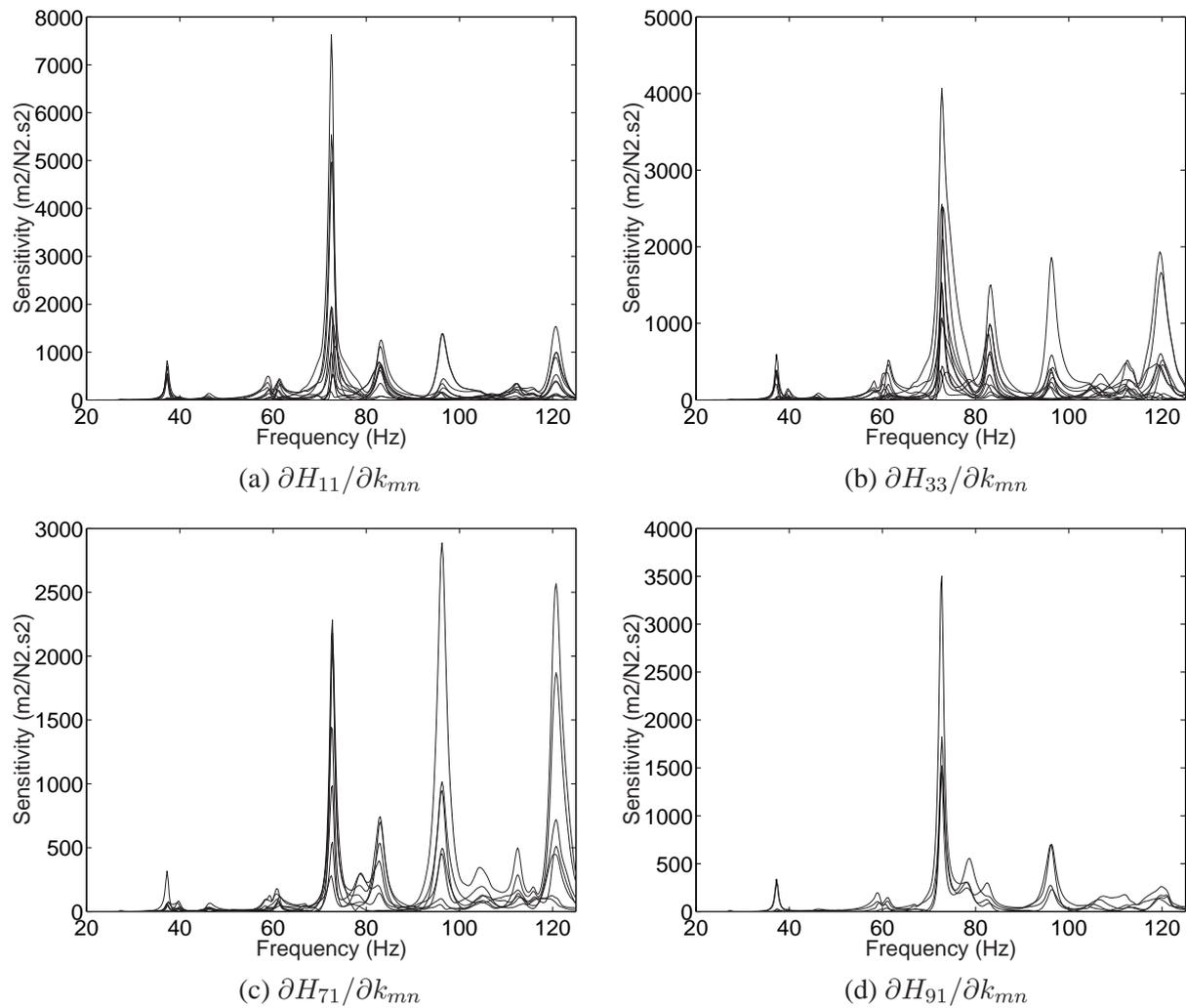
**Figure 5:** Embedded sensitivity functions of the four most important FRFs in the frequency range of 60 to 80 Hz.
