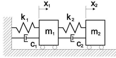
**Figure 1:** Analytical model of a two degree-of-freedom mechanical system.
